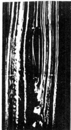
FIGURE 29.—Separation occurring on an airfoil at a low angle of attack.
