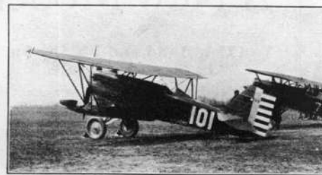
Side view of the scrappy Hawk. Note the N-struts, the shape of the wheels and the tail markings.
