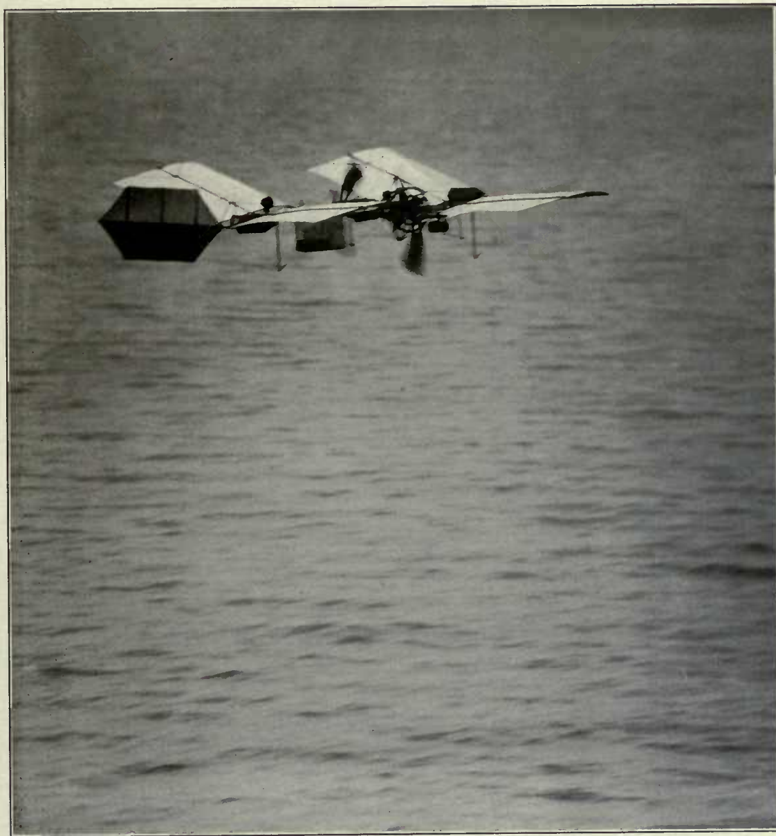
QUARTER-SIZE MODEL AERODROME IN FLIGHT, AUGUST 8, 1903
