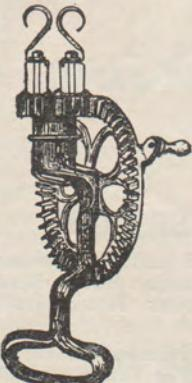
This is the regulation contest form of winder and is used for long distance flights where over 1,000 turns are required. (200 turns of the winder.)
