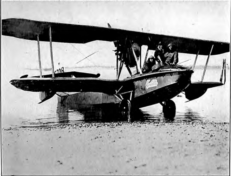
(Top) Hamilton Cabin Metalplane, Pratt and Whitney Wasp . (Bottom) Ireland Amphibian, Wright Whirlwind .
