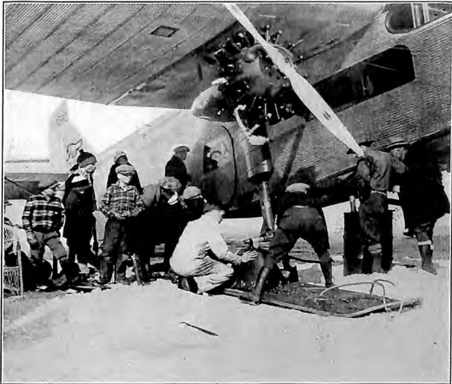
Installing skis on Ford transport for Byrd Antarctic Expedition.
