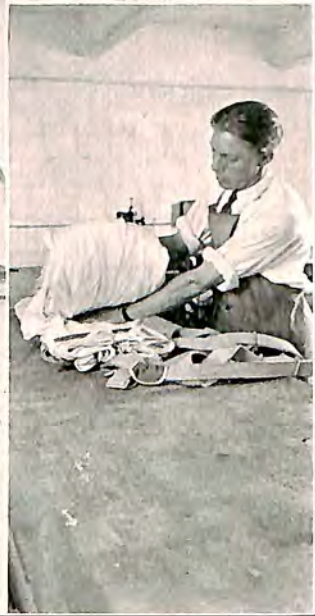
(Top) Pioneer Instrument Board. (Center) American Airports Corp. model of Mid-South Airport, N. C. (Lower Left) Heywood starter. (Lower Right) Folding Russell Lobe parachute.
