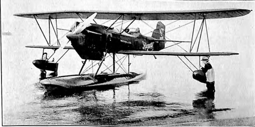
(Top) Curtiss P-3A Hawk taking off. (Center) Curtiss Falcon observation plane, powered with Curtiss Chieftain . (Bottom) Curtiss Falcon seaplane, Curtiss D-12 engine.
