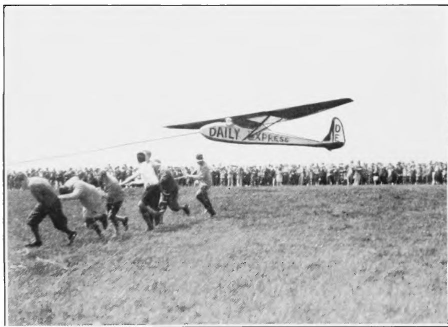
THIS PHOTOGRAPH SHOWS HOW A GLIDER IS CATAPULTED INTO THE AIR
