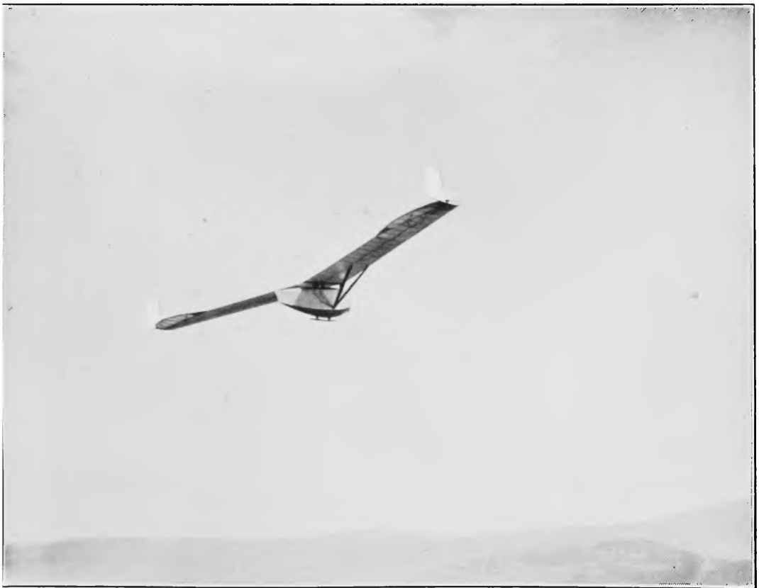
THE TAILLESS AEROPLANE "STORCH" AS A SAILING AIRCRAFT
