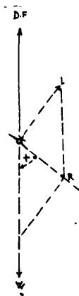
FIG. 78 D.F. Direction of flight L. Lift W Weight R Resultant sideslipping + Angle
