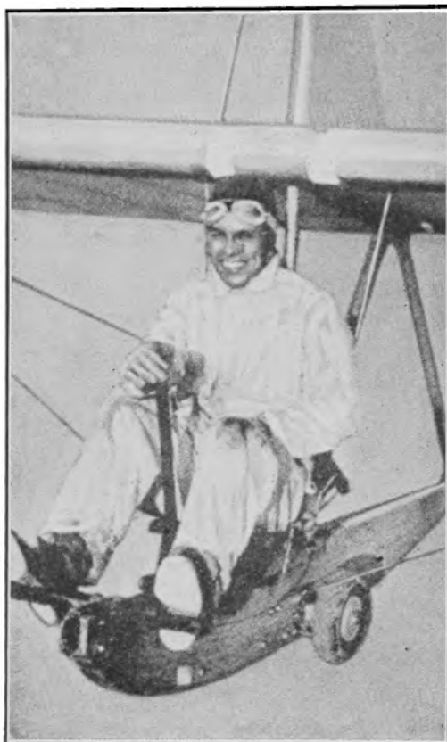
Fig. 33. —Partial Front View of Detroit Gull Training Glider Showing Pilot Seated and Simple Wheel Supporting Gear Employed for Launching the Glider by Towing with Automobile.
