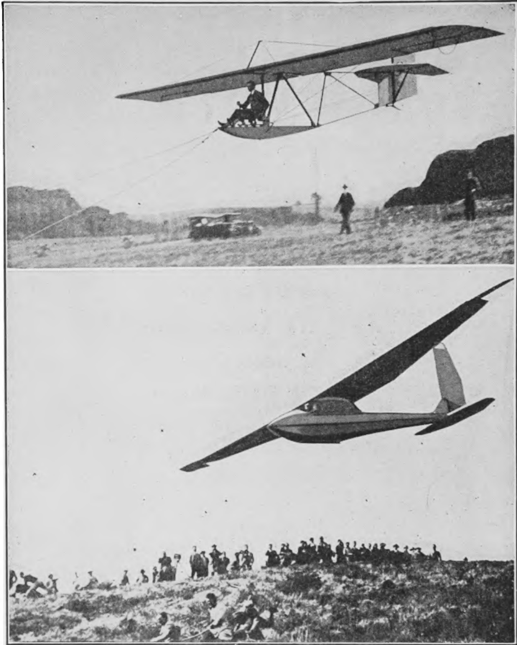
Frontispiece.—Illustrations Showing the Two Main Classes of Gliders. That at Top Shows a Primary Glider Launched by Shock Cord. The Bottom View Shows a Bowlus Sailplane, an American Built Soaring Type, in the Air.
