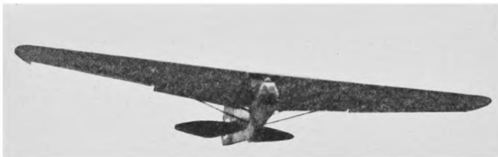
FIG. 64.—A secondary training glider in straight flight. The normal lateral and directional position of the glider in straight flight can be seen in this photograph.
