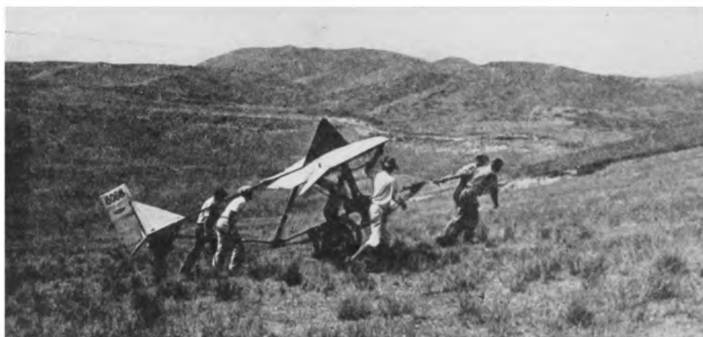
FIG. 77.—This means of transporting a glider requires less exertion. Here the weight of the ship is borne by the wheels upon which the fuselage is set.
