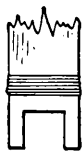
FIG. 33.—Manner in which the end of the brace can be bound with string to prevent splitting.
