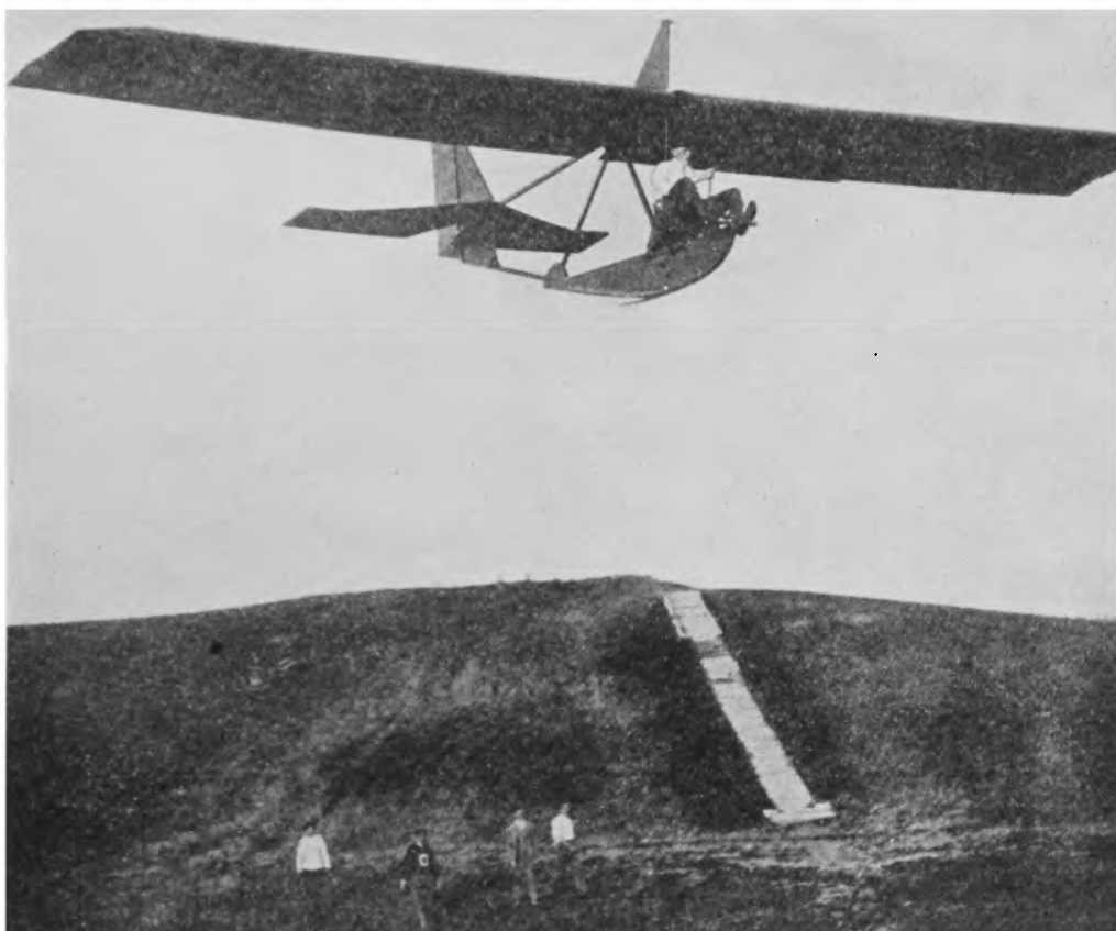
FIG. 9.—A glider in straight flight. This ship is flying straight ahead and not allowing one wing to drop below the level of the other. At the same time, it is gliding gently downward.
