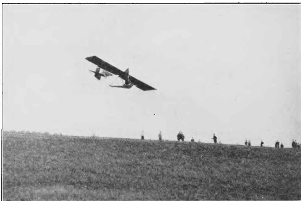
FIG. 78.—A bank. This glider is making a gentle left turn. By use of left rudder and movement of the stick to the left, the ship has been tilted into this bank. Note the angle of glide which insures the pilot against the danger of stalling.
