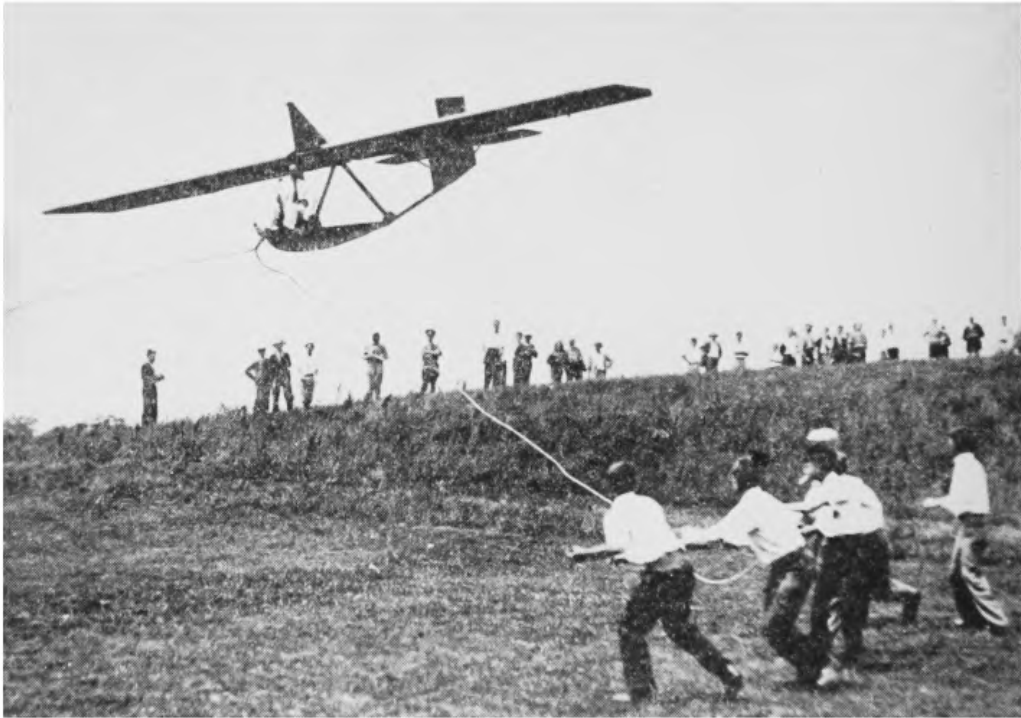
FIG. 8.—A take-off. This glider has just been launched by a rubber shock cord which works in the manner of a sling shot. The shock cord is tardy about falling off the glider's nose, and has begun to pull the ship down again.
