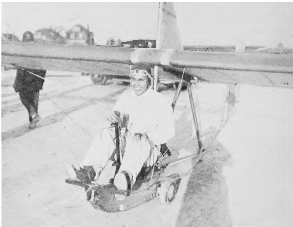
FIG. 5.—The controls. The rudder-bar and stick can be seen plainly in this photograph. The rudder-bar and stick are connected by wires with the control surfaces (the rudder, elevators and ailerons) which direct the ship's movements.
