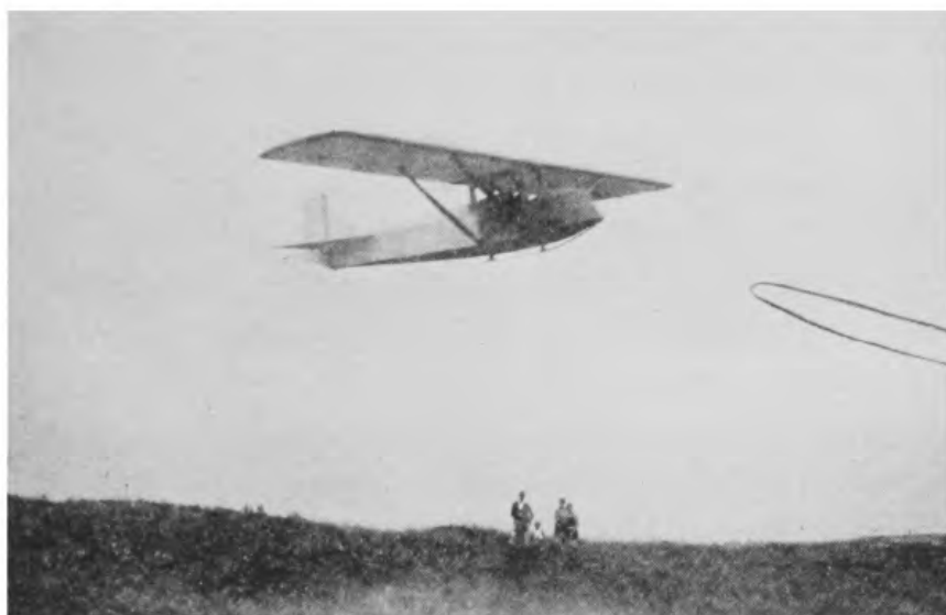
FIG. 61.—The shock cord falls off. Here the shock cord, no longer taut, has dropped from the hook on the nose of the glider. The pilot, at this altitude, is pushing the stick forward into neutral.
