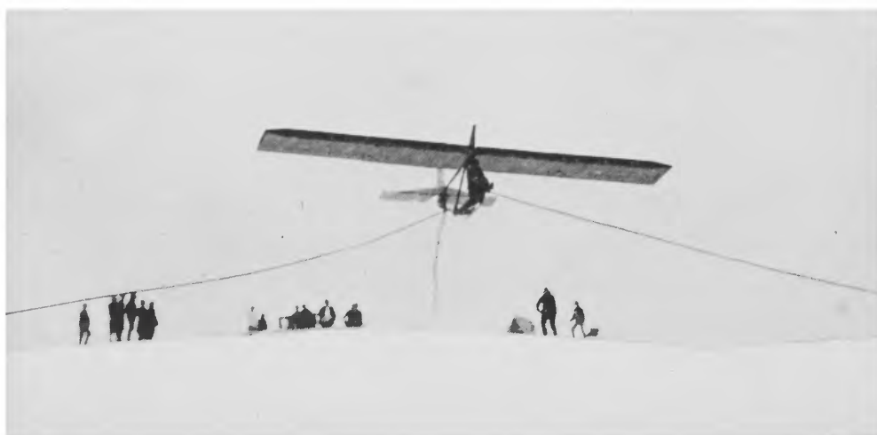
FIG. 66.—The climb. The glider has been shot into the air by the shock cord, and, at a good speed, is gaining altitude.
