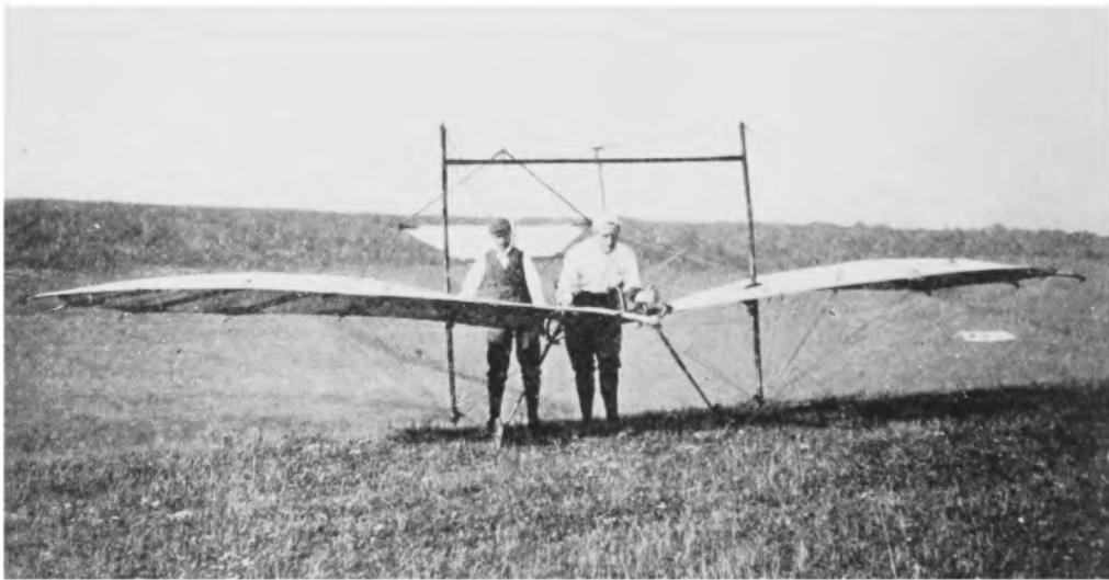
FIG. 13.—A glider built by Pilcher in 1897. This glider, of individual design, embodies the principle of cambered wing surfaces. It was the most successful of Pilcher's gliders, weighed 50 pounds, and once flew a distance of 100 yards.
