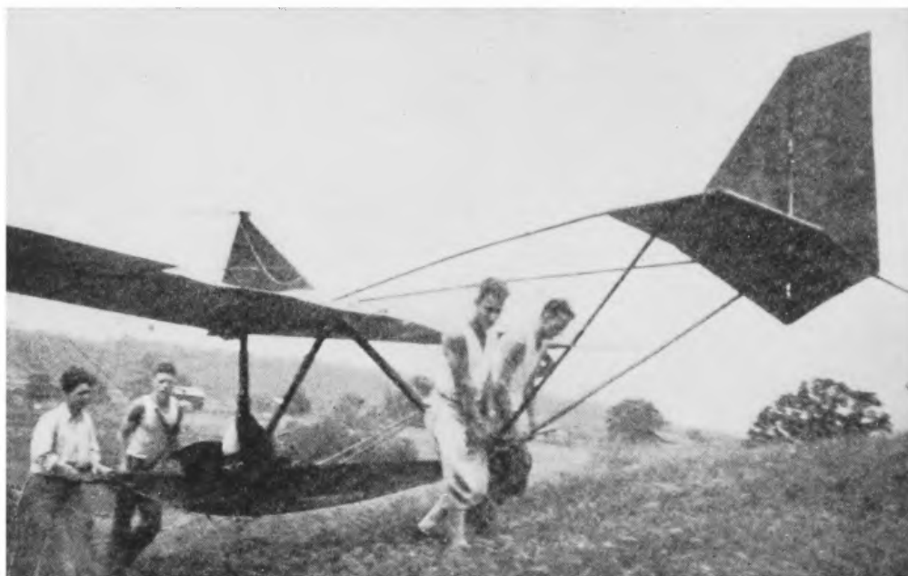
FIG. 76.—One method of carrying a glider uphill. This means is practicable only for a short distance.
