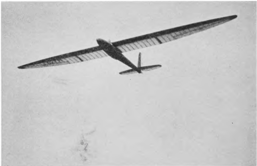
FIG. 44.—Another type of soarer. The broad span and perfect streamlining, which allow the soarer to stay aloft so long, are visible here. This glider was flown by the German flyer, Klemperer, in Pennsylvania, for 15\frac{3}{4} miles.
