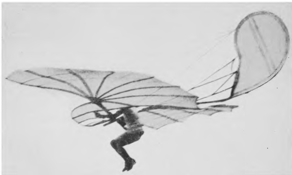
FIG. 11.—One of Lilienthal's gliders. This glider was built and flown by Lilienthal in 1894. In designing the bat-like wings, he utilized the principle that curved wings are more efficient than flat ones.
