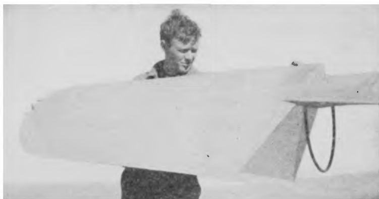
FIG. 53.—Lindbergh placing a wing-tip aileron on a Bowlus sailplane. This aileron is an unusual type.
