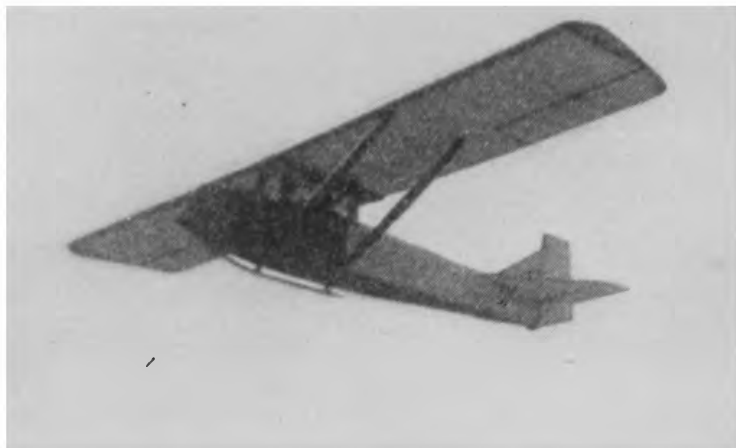
FIG. 40.—A secondary training glider. This glider is used by the student as soon as he has made a few flight attempts in a primary training glider. Although it will soar, it is less sensitive and more stable than a real soarer.
