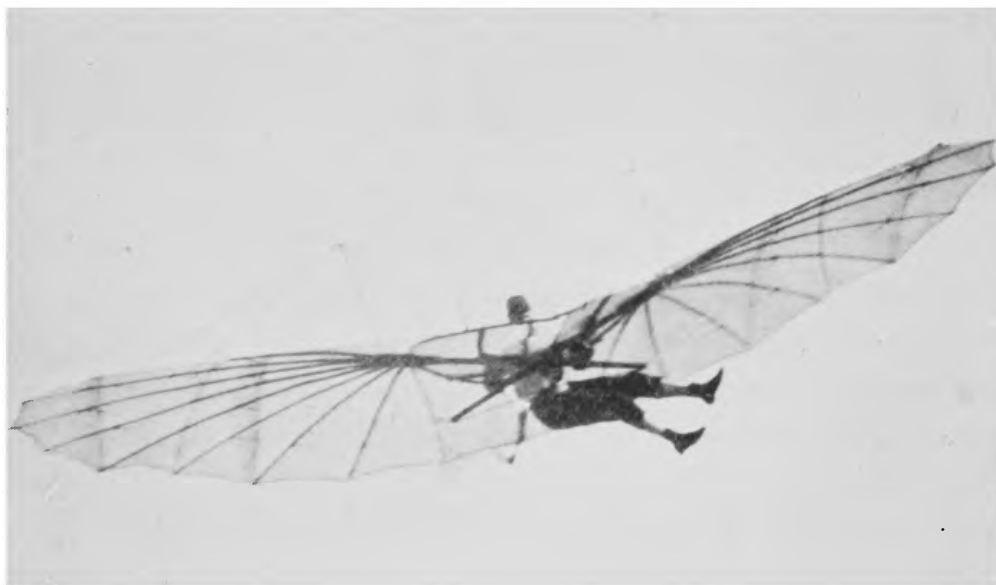
FIG. 12.—Another view of Lilienthal's glider. This photograph shows very plainly the way in which the pilot swung his body in order to bank the ship.
