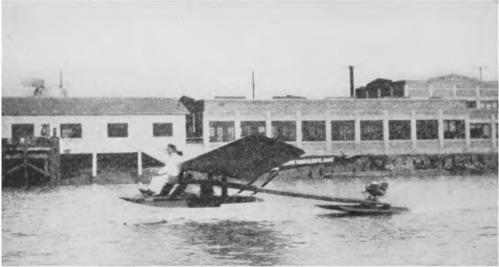
FIG. 90.—A waterplane in flight. This craft, propelled by an outboard motor, is a combination glider and speed boat. The wings lift the body of the ship high enough into the air to give the pilot some of the sensations of flight.
