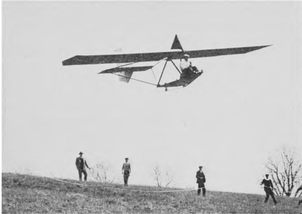
FIG. 10.—A turn. The pilot of this glider is using rudder and bank in order to effect the turn. The ship here is banked to the right, i.e. , the right wing is lower than the left, in order to offset centrifugal force in a right turn.
