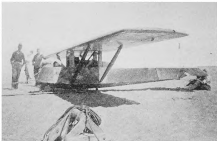
FIG. 59.—A side view of the glider in position for the take-off. Here the man can be seen who holds the glider stationary while the rest of the ground crew are running ahead with the rubber cable.
