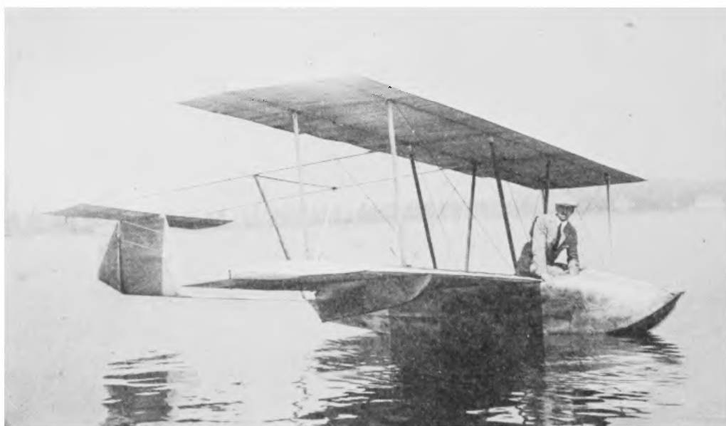
FIG. 6.—A water-glider. This glider is built with a water-tight hull, so that it will take off from and land in the water. Glenn H. Curtiss, the builder of the ship, is shown in the cockpit. Mr. Curtiss was one of the pioneers of aviation.
