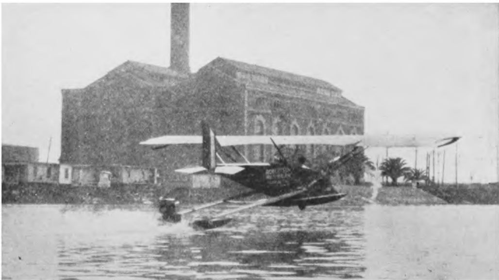
FIG. 91.—Another waterplane. The rudder of this ship is stable. But the ailerons and elevators provide the pilot with some opportunity of practicing the use of airplane controls.
