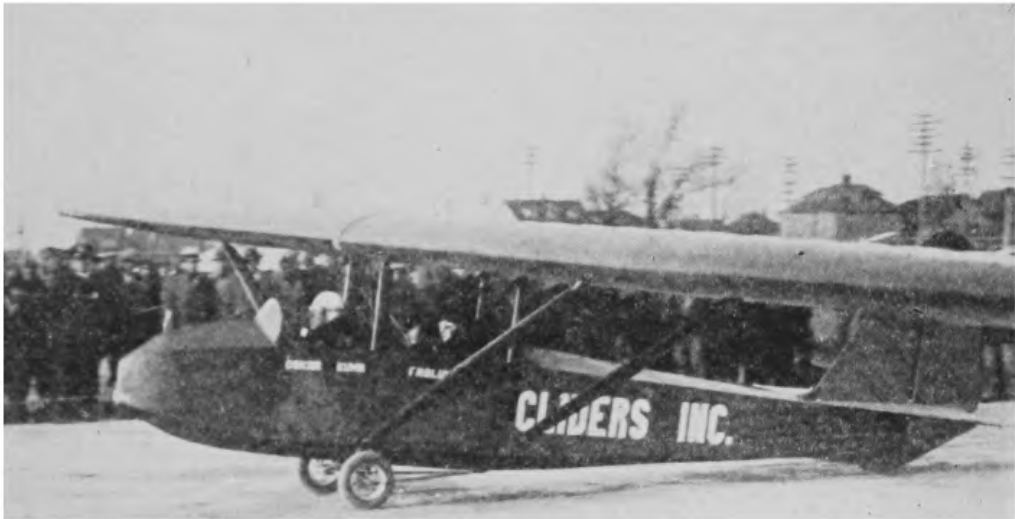
FIG. 7.—A two-passenger plane. In this glider both pupil and instructor may fly at once. Each cockpit is equipped with a set of controls, so that the pilot can correct wrong control movements made by the student. The pilot sits in front.
