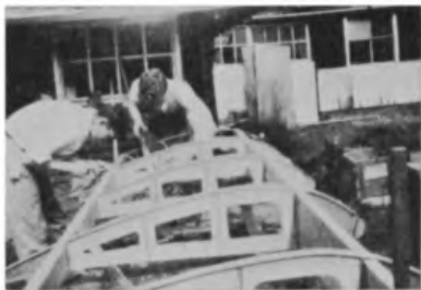
Ribs are threaded on to spars and secured with glue and screws.
