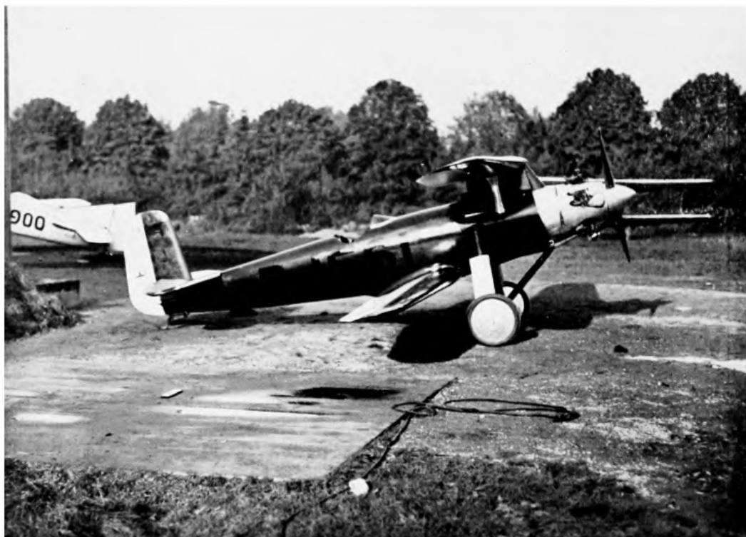
23. THE DARMSTADT ACADEMIC FLYING GROUP'S D.18. FUSELAGE AND WINGS SHOW THE EFFECT OF THE EXPERIENCE GAINED IN SOARING FLIGHT
