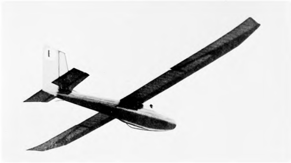
13. "KONSUL," THE MACHINE BELONGING TO THE DARMSTADT ACADEMIC FLYING GROUP. A PROTOTYPE OF THE MODERN HIGH-PERFORMANCE MACHINE WITH A WIDE SPAN
