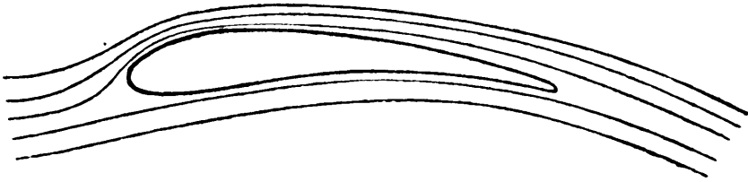
FIG. 6.—Airflow over Wing at Zero Incidence.
