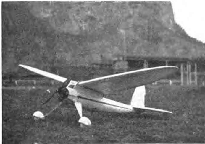
Fig. 99. The "Swallow", seen on the race-course below the "Rock" of Gibraltar. It is here fitted with a 4 c.c. Atwood "Phantom" engine.
