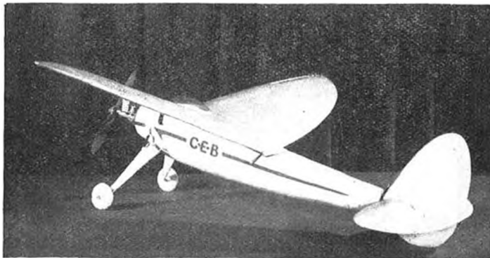
Fig. 86A. A small monocoque model built by the author and flown by a 1\frac{1}{2} -c.c. "Mills" diesel engine. The model flies very slowly and has a 43-in. span. Centre chord 10 \frac{1}{4} in.—wing tip slots are to be fitted. The fuselage is planked with \frac{1}{16} -in. thick planks.
