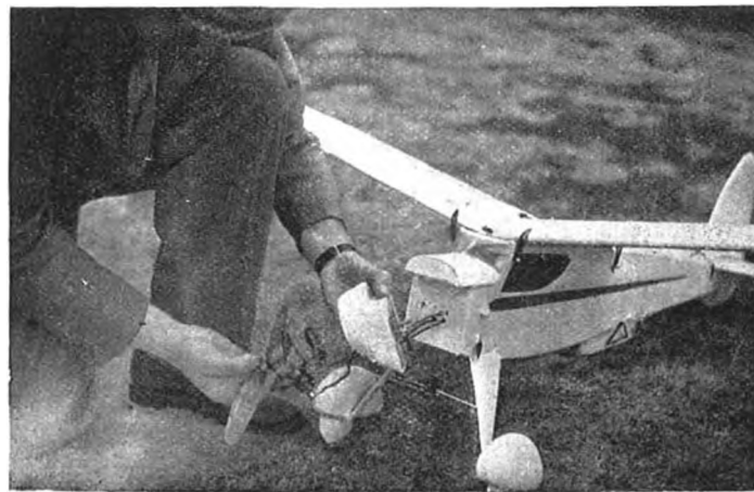
Fig. 14A. This type of square nose, designed by the author, allows a built up detachable nose with engine to be used, or the solid balsa distance-piece and Elektron casting as shown. By kind permission of Aircraft (Technical) Publications Ltd.
