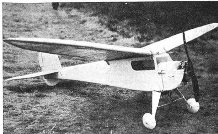
Fig. 14. A simple model by the author. In this case the detachable engine mounting is made from wood, and has the coil and battery mounted in it.
