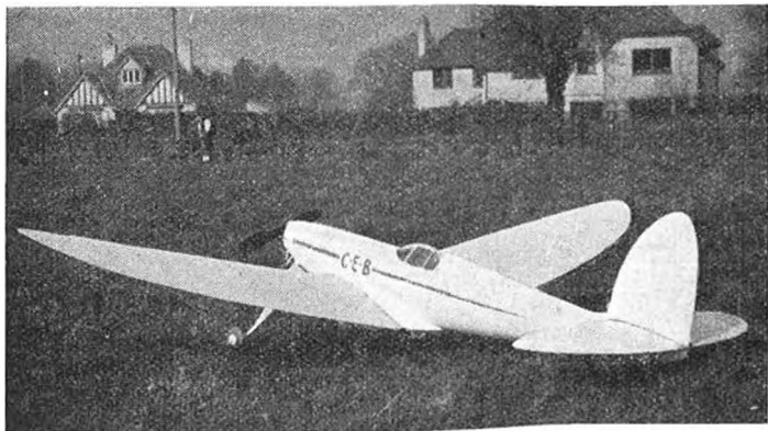
Fig. 105. The author's low wing semi-scale monocoque model "Mallard." The fuselage is balsa planked.
