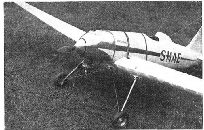
Fig. 55. A beaten-aluminium engine cowling is here seen fitted to an early 9-ft. span model built by the author.
