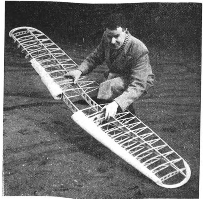
Fig. 64. A complicated, but interesting, wing. The trailing edge is weak.
