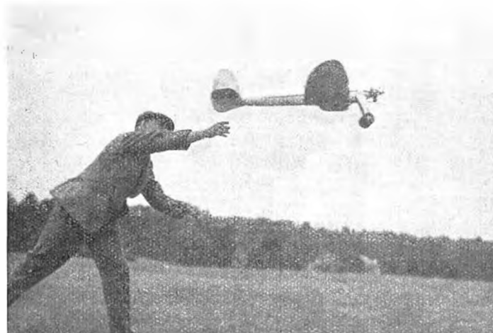
Fig. 135A. The author hand launching the small monocoque petrol model shown in Fig. 51A, on page 110.
