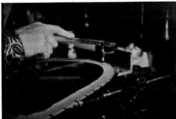
FIG. 119. Cutting slots for the long- erons in a 3-ply bulk- head, as described at foot of the pre v i o u s page.
