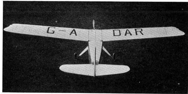
This 8 ft. span high-wing petrol 'plane, designed and built by the author, made many successful flights in 1939.
