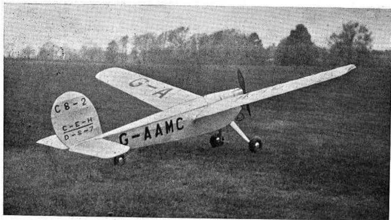
This shoulder-wing petrol plane, designed and built by the Author, is of 7 ft. span, weighs 6 lb., and is powered by a 6 cc. "Baby Cyclone" engine. It is of fairly typical design to the aircraft described in Figs. 10 and 11.
