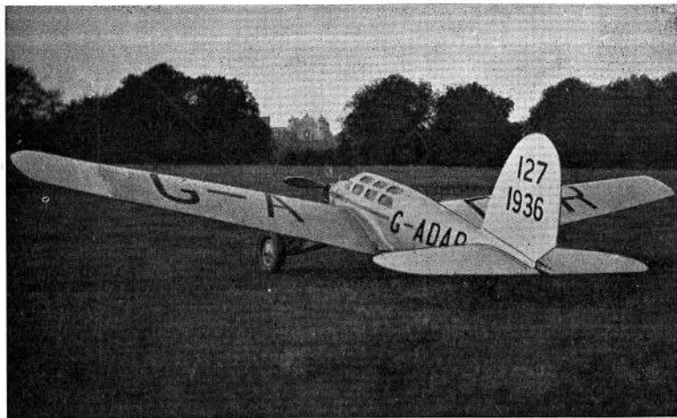
At the time the author built this low-wing monoplane of 10 ft. span it was one of the largest, and certainly the heaviest, of models to be built. The span of the 'plane is 10 ft., and the weight is 14 lb. The model is powered with an 18 cc. "Comet" engine, and it was awarded a "Highly Commended" diploma at the Model Engineer Exhibition in London, 1935. The 'plane was also awarded first prize at The Concours d'Elegance at the Northern Rally, organised by the Lancs M.A.S. in Manchester in 1936.
