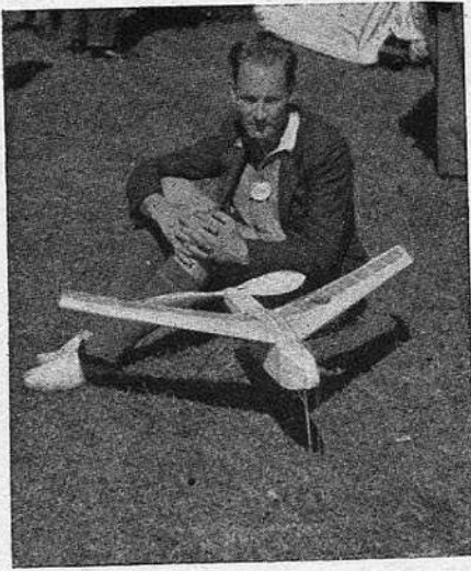
Here is Mr. Howard Boys with two tail-less models of his own design. They hold the British records in their class, one for hand-launched flight and the other R.O.G. Mr. Boys successfully treats his scale models very much like tail-less machines for stability, the idea being that a very small tail-plane is little better than none.
