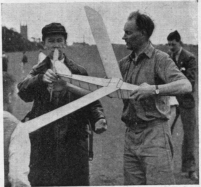
Here is Mr. Howard Boys with two tail-less models of his own design. They hold the British records in their class, one for hand-launched flight and the other R.O.G. Mr. Boys successfully treats his scale models very much like tail-less machines for stability, the idea being that a very small tail-plane is little better than none.
