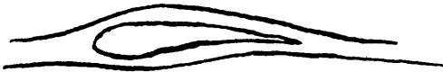
FIG. 6.— The curved airfoil showing the airflow around it. This gives much more lift than the flat wing.
