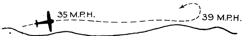
FIG. 31.—This shows the correct way a turn should be made at the end of the soaring ridge. It will be noted that the speed is increased from 35 m.p.h. to 39 m.p.h. during the actual turn. The importance of this cannot be overstressed to new pilots.
