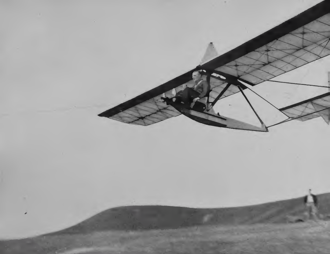
Top: The first stage of a primary "bunje" launch. Bottom: The second stage. The rope is about to fall clear.
