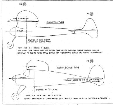
As a safeguard against stalling a temporary downthrust packing equivalent to about 5 degrees, can be installed on the motor mount.
