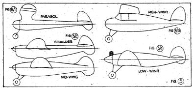
The tailplane should definitely be rigged to carry part of the load on a parasol model. Authorities differ as to how far aft the C.G. can be located with safety, but the writer favours a position 50 per cent. of the average chord; never further aft than 66 per cent. of the average chord from the leading edge. Similar rigging may be adopted on high wing models, although the "non-lifting" tailplane is here less tricky, i.e., rigged as in 3/1 or 3/2.
