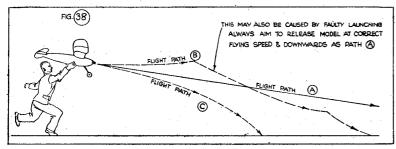
The model may also be trimmed by the tailplane, increasing the tailplane incidence *slightly* to cure the stall of flight path B, and decreasing the incidence *slightly* for flight path C. However, this method of trim is more liable to abuse and is not recommended to the beginner.
