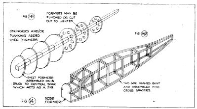
Suitable material sizes for any new design are best decided by reference to plans of previously successful models. As a guide to crutch member sizes:  $1 \times \frac{3}{16}$  spruce or birch is suitable for large models;  $\frac{1}{2} \times \frac{3}{16}$  spruce for medium sized models;  $\frac{3}{4} \times \frac{1}{4}$  hard balsa is also suitable for medium sized models;  $\frac{1}{2} \times \frac{3}{16}$  balsa for smaller types and  $\frac{3}{8} \times \frac{3}{16}$  balsa for baby models.
