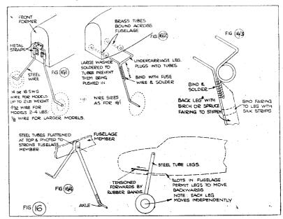
The American system is simply to employ a wire cantilever unit bolted or sewn to the nose former of the fuselage (invariably of plywood on *all* petrol models)—see Fig. 16/1. The size of the wire chosen depends upon the weight of the model, typical diameters being indicated on the diagram.
