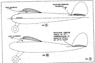
This is rather cumbersome to use and the simple approximation of one-half the wing incidence is more convenient for the average designer. The correct tailplane rigging angle can also be found by test-gliding as detailed in a later chapter.
