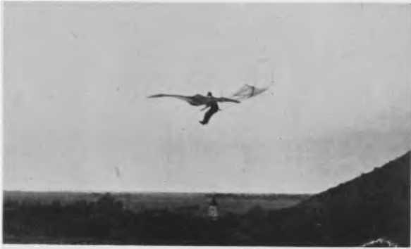
Fig. 1. Otto Lilienthal flying his monoplane glider (about 1893). Note the slope of the hill, the glider's angle of descent is almost as steep.
