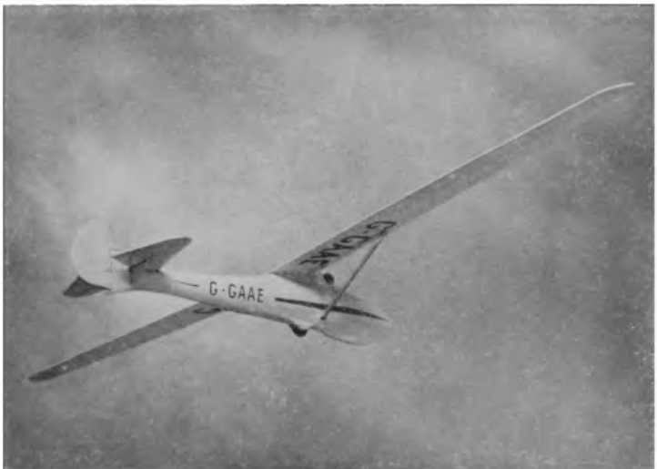
PLATE 9. The Kite II, Britain's first post-war high-efficiency sailplane. Gliding angle is 1 in 22. Rate of sink, 2.2 ft. per sec.
