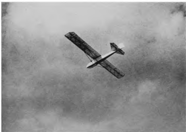
PLATE 5. The Cadet, a secondary training aircraft suitable for ridge soaring. Its gliding angle is in the neighbourhood of 14 to 1.
