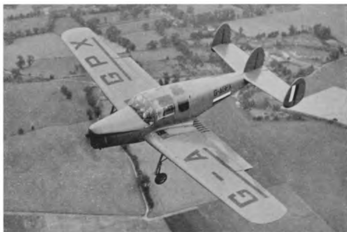
PLATE 17. Miles Messenger, a modern four-seater passenger aircraft suitable for training. When the author flew this aircraft, he reduced speed to 28 m.p.h. before she stalled.
