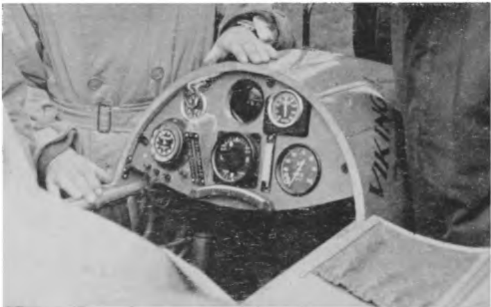
PLATE 11. Instrument board of the Viking. An electric turn and bank indicator makes cloud flying a practical proposition.
