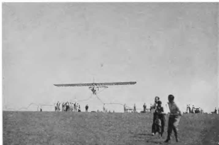
PLATE 4. The crew on the elastic launching rope have done their work. The primary glider with its pupil takes off for a "low hop."
