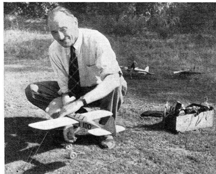
Fig. 14—Mr. Cathcart getting his mixture right with rapid and practiced hands prior to a control line flight with a "Frog 160" glow plug engine.
