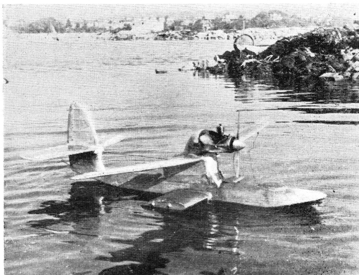
Fig. 39—Try your hand at control line flying from water. It can be done from the bank or shore of a pond or the sea. This model is fitted with an E.D. glow plug engine, and was made by the author.
