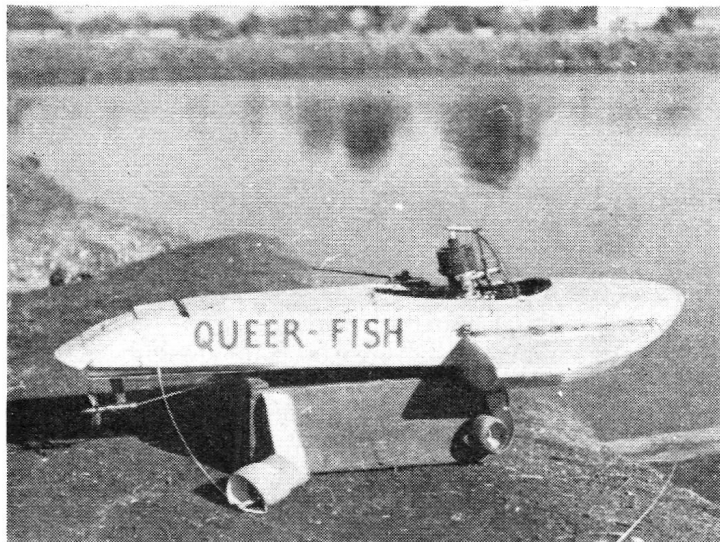
Fig. 34—The author's "C" class three point suspension hydroplane is now run on glow plug ignition to lighten the planing load.
