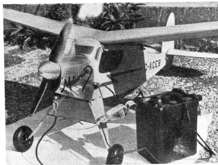
Fig. 12—The author's Meteorite model fitted with a British glow plug that can safely take a 2-volt accumulator for starting.
