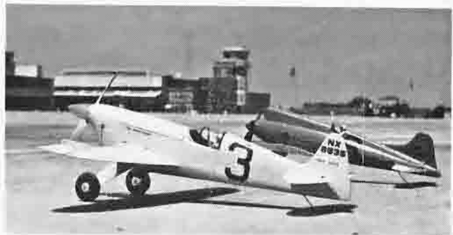
● Two semi scale racers by Les MacBrayer (No. 3) and Keith Storey—of the Los Angeles FAST club. Motors are K & B Torpedo in No. 3 and McCoy 29 in No. 6.
