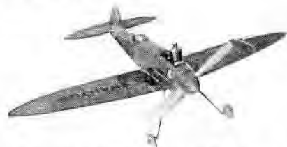
● PHANTOM—Well-known C.L. trainer. All sheet construction is popular with this type of model.
