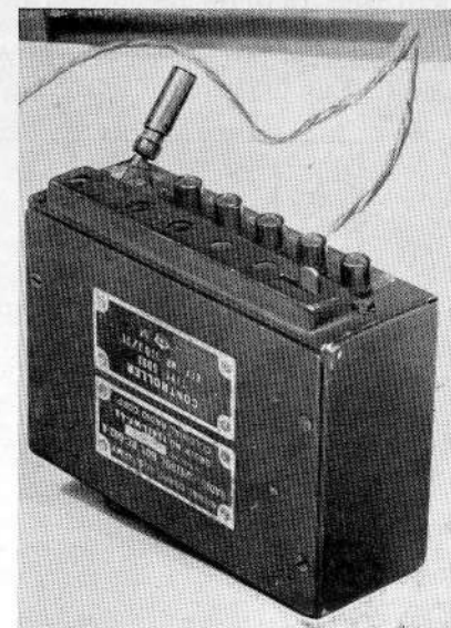
A very handy type of control box of ex-Forces origin. The lever switch is for rudder control, the push buttons for the auxiliary controls.
