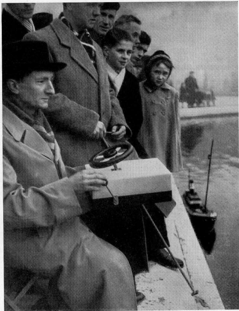
The outstanding L.U.K. team transmitter, operated by one of its designers. The box contains transmitter, batteries, controls and internal frame aerial. The large wheel operates a progressive "following" rudder, the lever giving forward, reverse, stop and start, including half speeds. The positions make it child's play to operate, lever right forward=full speed ahead, half forward=half speed ahead, centre=stop, and the same movements in reverse. This equipment was the well-deserved winner of the Miniwatt international competition, 1949, in France. Alongside is the R.C. steam freighter of C. Pepin.
