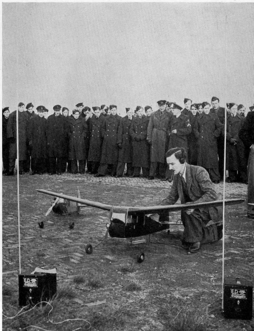
The author checking his equipment prior to a demonstration before members of the Dutch Air Force. The model shown is one of the well-tried Electron series developed in various sizes as flying test beds for new equipment.
