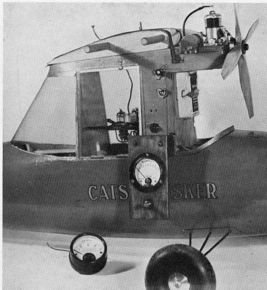
General arrangement of receiver, batteries and engine on this model designed and built by Squadron Leader E. D. Cable could hardly be bettered. Adequate access to the "works" is given without in any way weakening the basic fuselage, and extreme forward position of H.T. and L.T. batteries prevents them from damaging radio equipment or wiring should anything go amiss. Last minute adjustment can also be made with mainplane in position—a matter not always considered.
