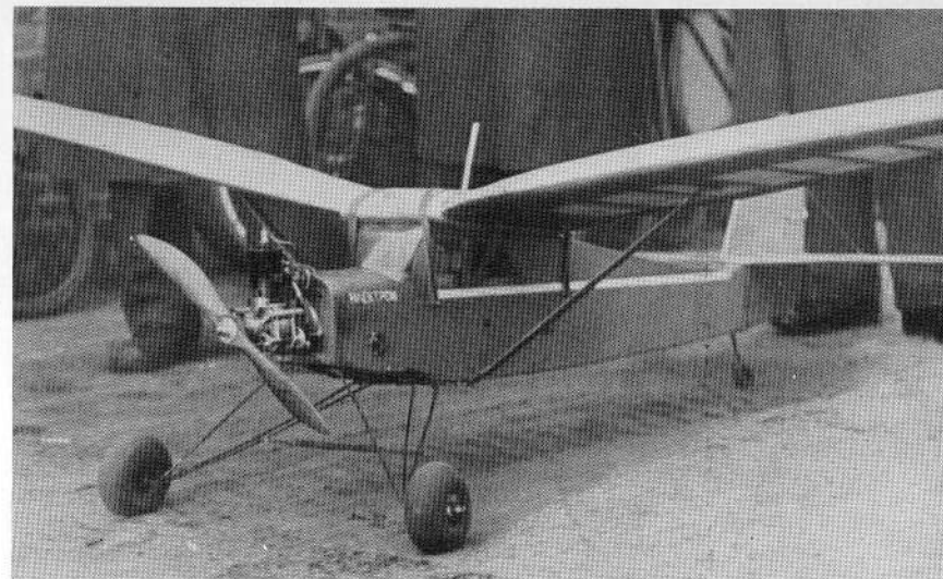
An early "test bed" for experimental radio receivers. 15 c.c. Magpie engine, 72-in. span, rear wires of undercarriage sprung in slots.
