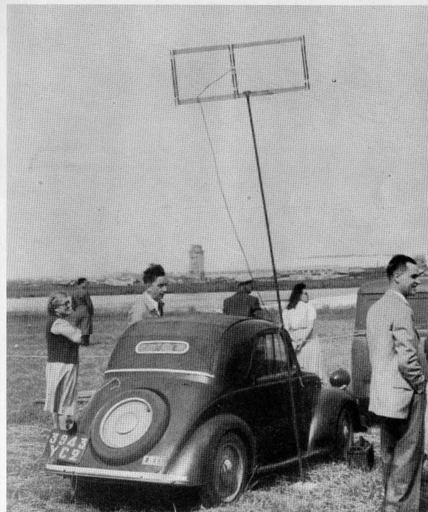
Aerial array used by French postal authorities to check frequencies at the 1949 International Competition. A half wave dipole with both reflector and director.
