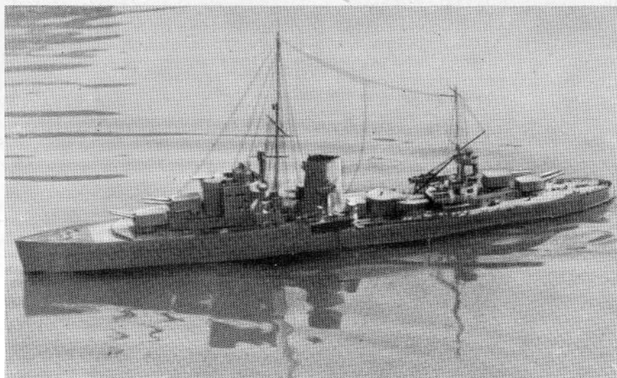
H.M.S. Ajax. A perfect scale model by F. H. Mitchel. Powered by twin electric motors and operated by E.D. R.C. with delayed relay reverse, it might well be the real thing.
