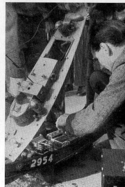
(Top) Tail of Electron 6, showing easily adjustable rudder horn. Note slight angle of pin for free movement in loop at right angles.
