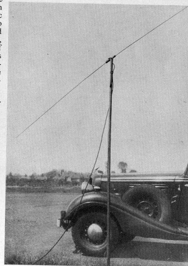
The Author's half wave dipole aerial used on tests for the French 72 MC band. Field strength tests however showed that over the visual distance of model control, the vertical quarter wave aerial was hardly inferior.
