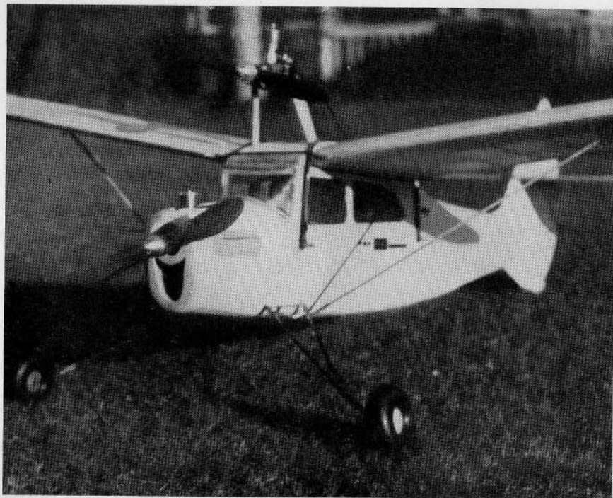
The author's "Eros" twin engine. The smaller high wing engine, E.D. Competition special, was used as a boost to aid initial climb with only a small fuel tank. The main engine, E.D. Mk. III, then had ample power to maintain height for scale type maneuvers.
