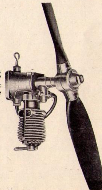
Fig. 32. The "Frog 180" has a larger capacity than the "100." Bare weight is 3.75 oz., static thrust 20 oz., 10 in. diameter adjustable pitch airscrew fitted.
