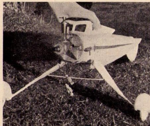
Fig. 14. Testing the installation and running the engine on the fuselage, whilst the wings and tail are being made.
