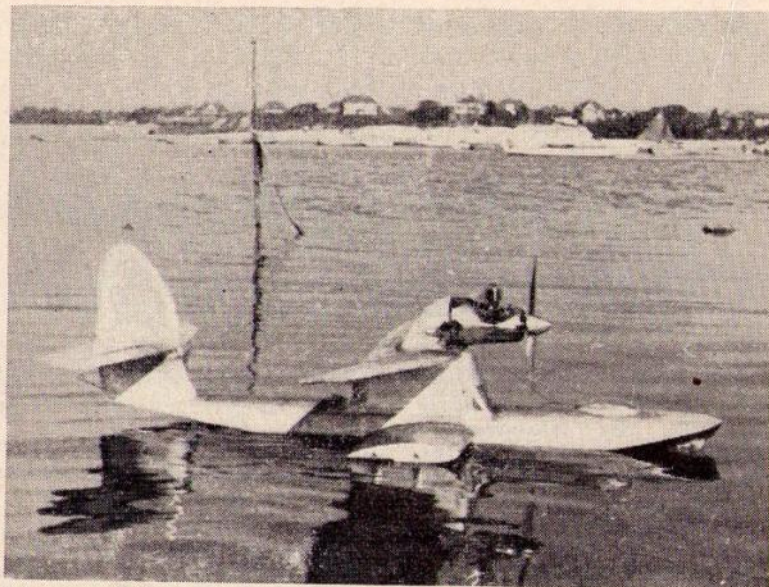
Fig. 113. The author's control line flying boat, which successfully takes off and lands on water with the operator standing at the water's edge. A special forward fin is required to resist the inward pull of lines at take-off.
