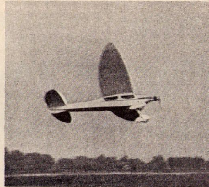
Fig. 120. The author's "Whitewings" is turning to the left under radio control. The nose is held up by area low down due to spats and filled in undercarriage legs, which act as forward keel.
