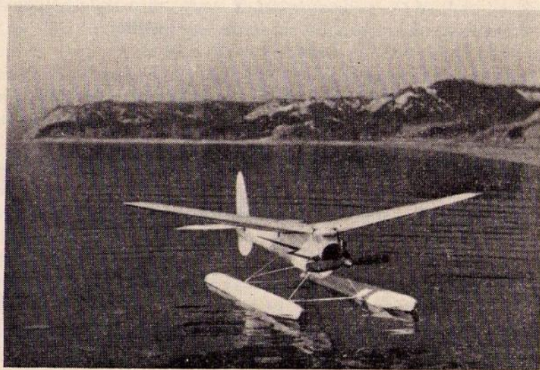
Fig. 100. The author's 2.4 c.c. E.D. diesel powered monocoque twin-float plane flies with remarkable stability. Span 48 in.
