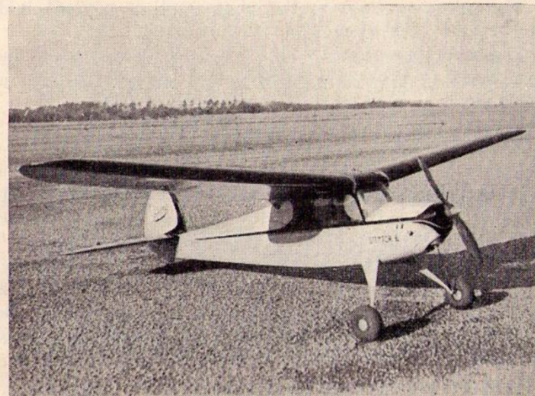
Fig. 107. Mr. P. Smith designed this nice-looking 7 ft. span "Stentor 6," fitted with parallel chord wings. A number of these models have been fitted with radio after slight modification.
