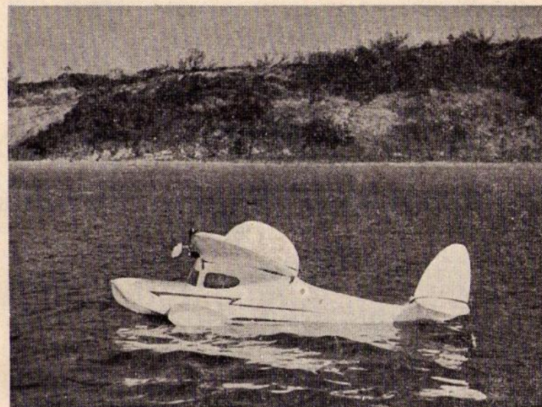
Fig. 94. The author's 48 in. span cabin flying boat designed for 2.4 c.c. diesels such as the "Elfin." Suitable for radio control with a baby receiver in the cabin.
