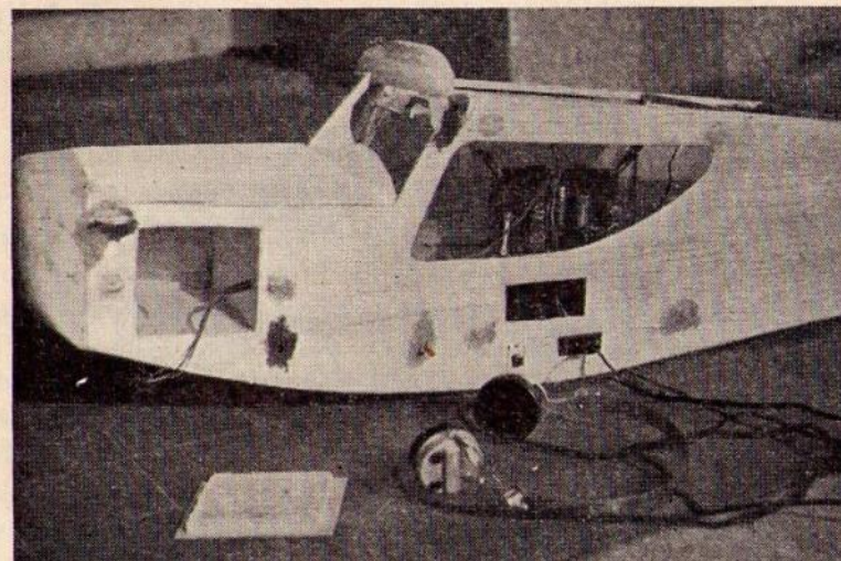
Fig. 124. The author's layout has a forward battery compartment with receiver and servo behind. The receiver is held in position by rubber bands to four cross members in the fuselage. The white tuning arm on the receiver is reached by forefinger through opening in fuselage side. Below are main switch and tuning socket for headphones, or meter.
