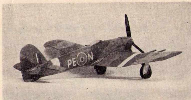
Fig. 112. Mr. "Natznees" Norman flies a scale "Typhoon" under perfect control at the "Bowden Power Trophy," 1948, by pendulum control to scale elevators and ailerons. The model was powered by a "Frog 100" diesel and flew as if a pilot who understood speed was at the controls. The ailerons and elevator sizes can be seen in the photograph of the model, which has a wing span of only 3 ft.
