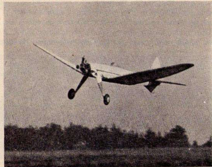
Fig. 90. The author's simple low-wing free-flight model is here seen flying with a 2.5 c.c. diesel.
