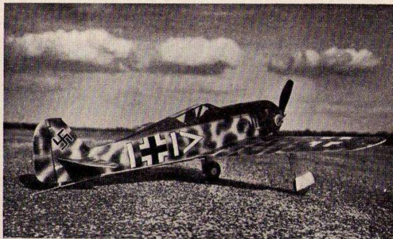
Fig. 85. Another Smith control line model is the Focke Wulf 190, A3, powered by a Mark IV, 3.5 c.c. diesel. Note the trailing edge flaps on the mainplane which go down when the elevator goes up, to assist quick stunt work.
