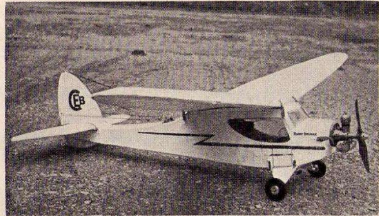
Fig. 82. The new "Hivac" valve radio sets encourage small radio models powered by diesel engines. The author designed his 48 in. span "Radio Brumas" for the latest lightweight radio sets. Engine is a 1.8 c.c. "Elfin."
