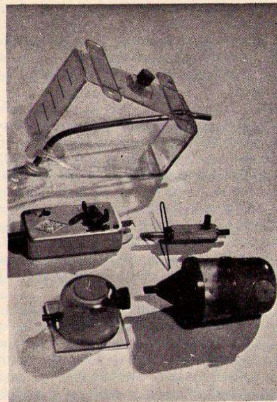
Fig. 59A. Useful Fuel Accessories. At top the large E.D. tank with graduated fuel level marks for radio flight of long duration. Note the well at lower corner to retain even flow when stunting. In middle, the E.D. clockwork timer to operate a switch on the F.G. fuel cut off seen beside it. Below two very useful plastic tanks for free flight and control line flying
