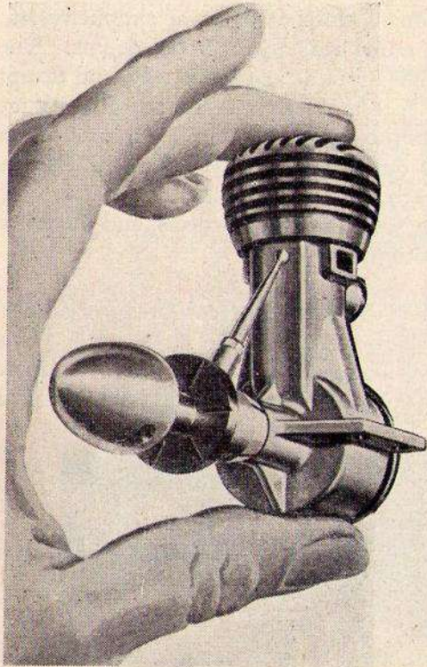
Fig. 39. The new "Airstar" of 2.147 c.c. has adjustable compression by means of the lever seen behind the propeller boss, which alters the crankshaft bearing mounted on an eccentric. The height of the motor is only 3\frac{1}{4} in., and it has a number of unusual features, including a fixed jet and adjustable air supply.
