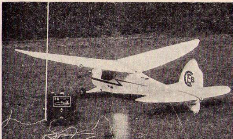
Fig. 127. The complete set up can be seen in this photograph. The rudder tab is attached to the fin by fabric hinges like the elevator of a control line model.
