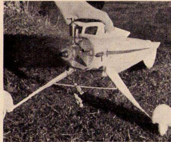
Fig. 14. Testing the installation and running the engine on the fuselage, whilst the wings and tail are being made.
