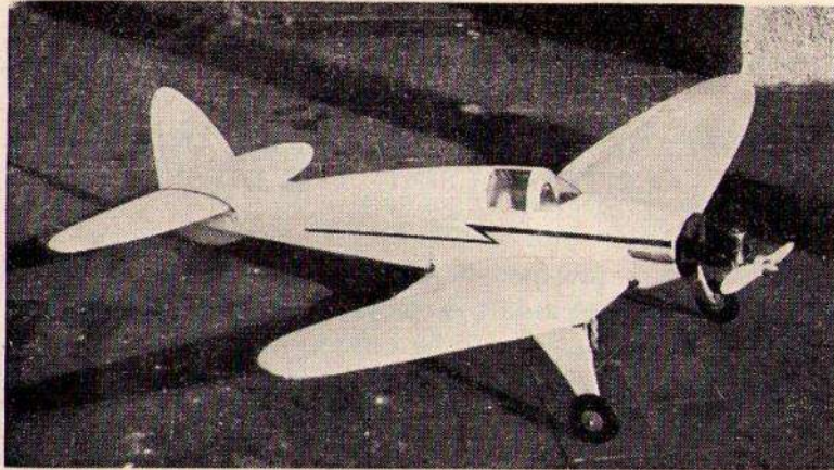
Fig. 77. The author's free-flight cabin low wing monoplane for 1 c.c. diesels.
