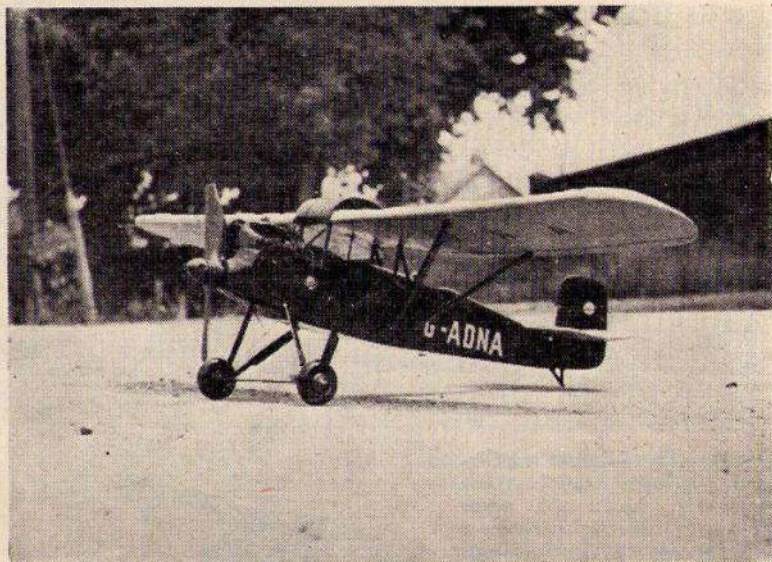
Fig. 79. This tiny control-line model of 17 in. wing span has flown successfully, powered by a "Kemp" 0.2 c.c. diesel. It is a scale model of a "Westland Widgeon."
