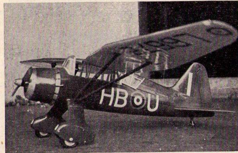
Fig. 76. Metal spinner and cowlings can be made from aluminium spun or beaten into shape. The cowling on this lovely flying scale "Lysander" adds much to its realism. The motor is a 2.4 c.c. E.D. diesel.
