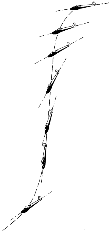
FIG. 167. WHEN THE DROP OF LIFT IS THE SAME ON BOTH WINGS THE SAILPLANE WILL DROP ITS NOSE AND START REGAINING SPEED AS SHOWN IN THE PICTURE
