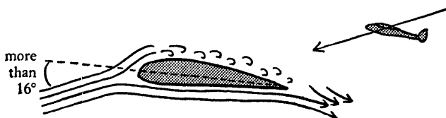
airflow over stalled wing
