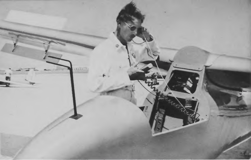
8. Radio maintenance: airbrakes and pitot head can also be seen. Corkscrewing through the Spanish sierras: a Sky trailer on tow.
