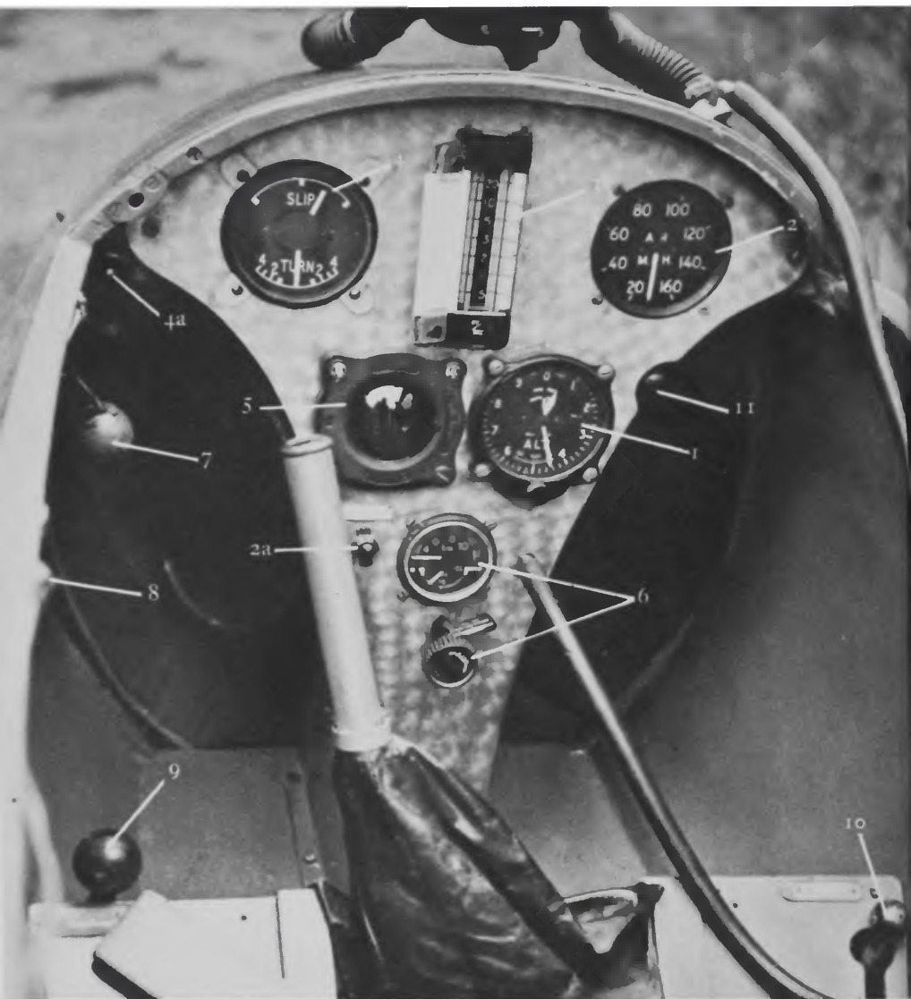
6. Instrument board: 1, Altimeter; 2, Air-speed indicator; 2a, Pitot head heater switch; 3, Variometer; 4, Turn-and-Bank indicator; 4a, Turn-and-Bank indicator switch; 5, Compass; 6, Oxygen; 7, Quick-release knob; 8, Airbrake lever; 9, Undercarriage release knob; 10, Tail-trim lever; 11, Ventilator knob.
