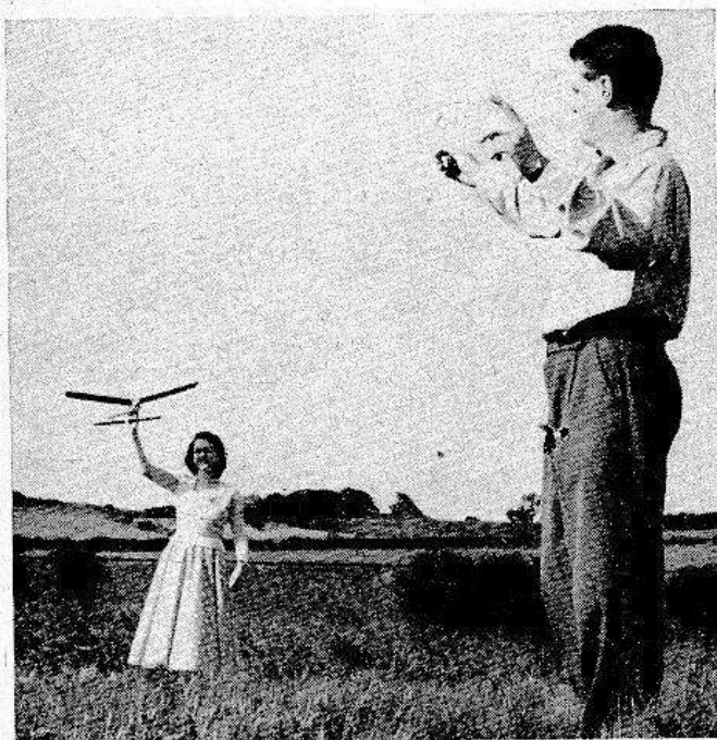
Fig. 9 (below). Ready for the start of a towline launch. Note how the operator is indicating to his helper that he is ready to proceed.
