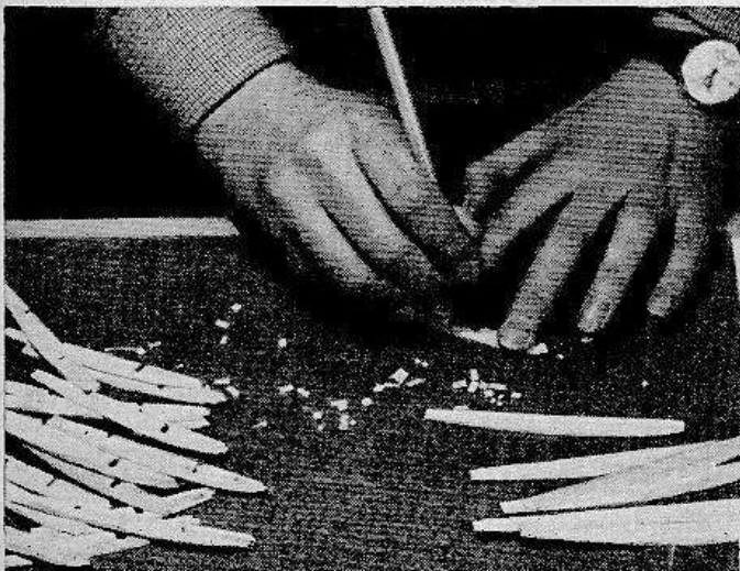
Fig. 1. Using a chisel-point knife for cutting spar slots in ribs.
