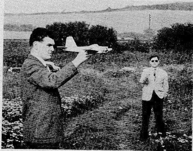
Fig. 5. With the aid of a helper, the pilot should check the controls for free movement and correct centring.
