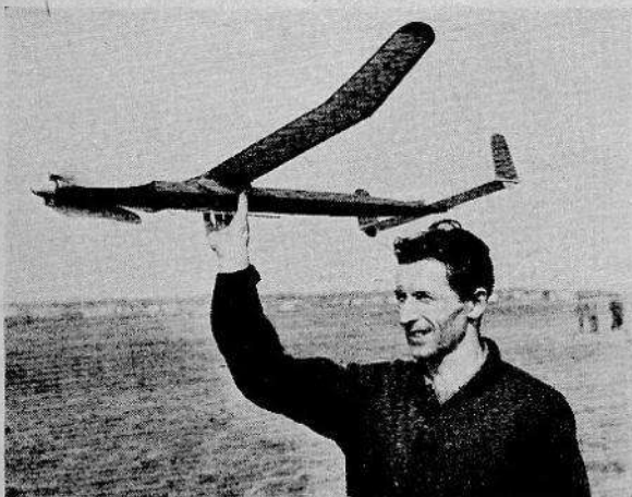
A typical modern rubber-driven competition model. Note the folding propeller. Built by Czechoslovakian enthusiast, V. Kutil.
