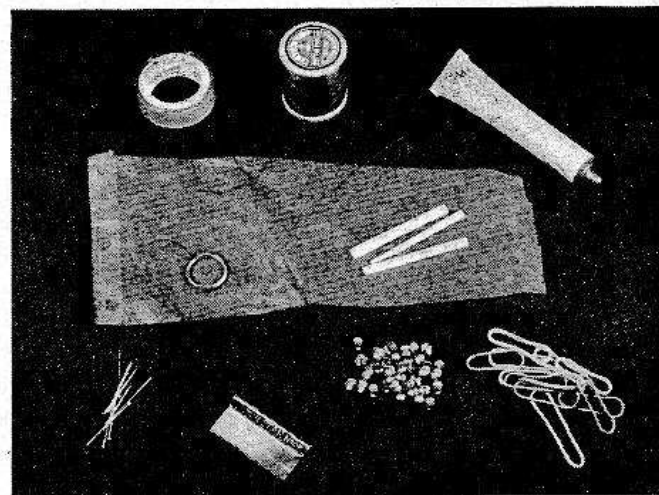
Fig. 4. A simple field kit: cellulose tape, button-thread for tow-line, cement, coloured tissue pennant, towing ring, thin strips of balsa for incidence packing, pins, razor blade, lead ballast and rubber bands.
