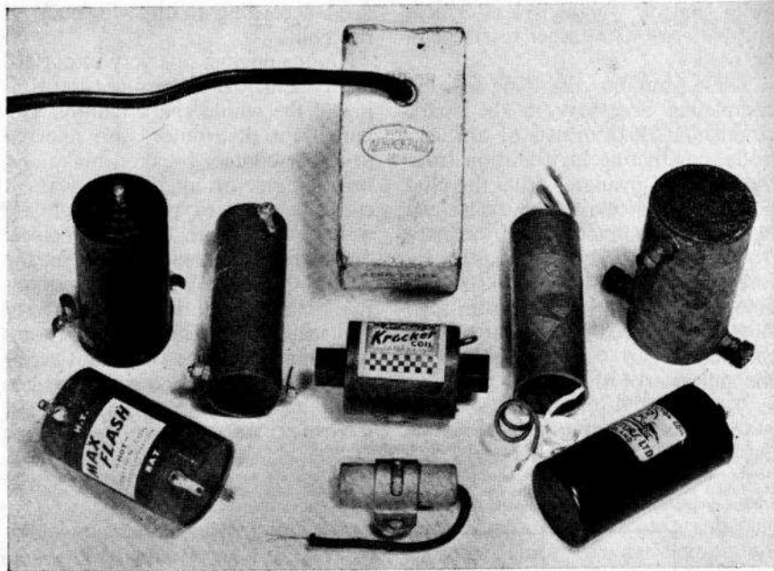
THIS ASSORTMENT OF COILS AND THE CONDENSER IN THE CENTRE FOREGROUND illustrate the diversity of shapes and approaches to the principal item in the petrol ignition circuit, some coils have plastic insulated casings, others are encased in a fibre tube.
