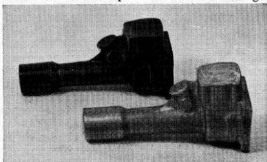
PATTERN FOR THE SUGDEN Special crankcase is carved in balsa, doped and polished. Sand casting obtained from it is in foreground. Similar gravity die-cast crankcases can be bought for 8/- through Aeromodeller Plans Service.
