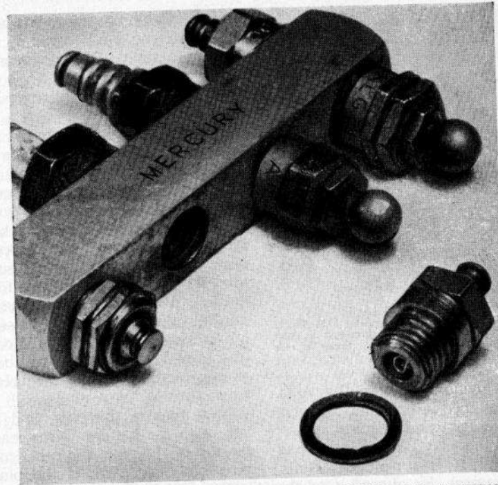
LARGER THAN LIFE PHOTO OF ASSORTED BRITISH AND AMERICAN glowplugs illustrates the diversity in design of the head connections. Nearest plug in holder is an Ohlson, extremely squat whilst those with spherical tops are KLG, the popular British make which has achieved great international reputation. Detached K & B plug in foreground shows the platinum-iridium wire coil and copper gasket.
