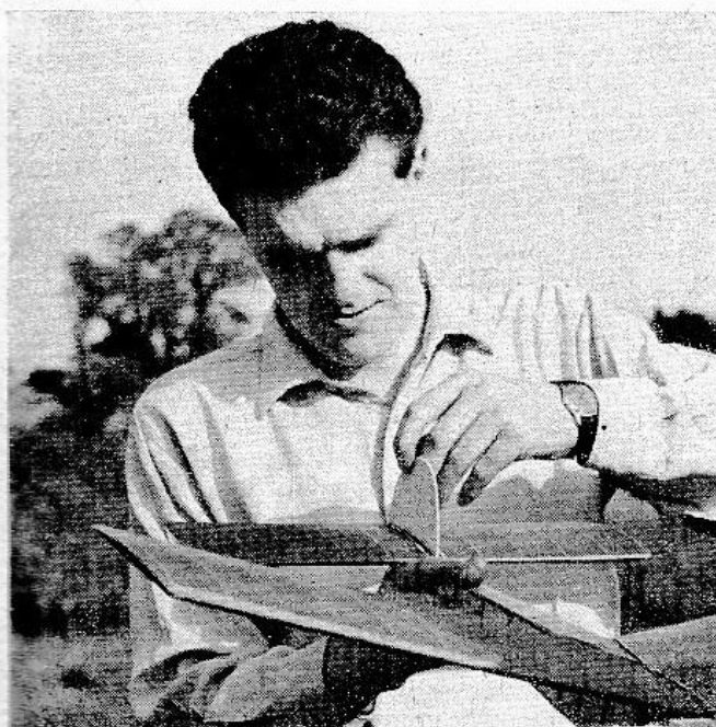
Fig. 7. Any tendency for the model to veer left or right can be corrected by slight adjustments to the rudder tab.
