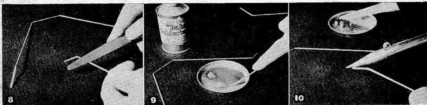
Figs. 8-10. Cleaning and tinning wire undercarriage parts.
