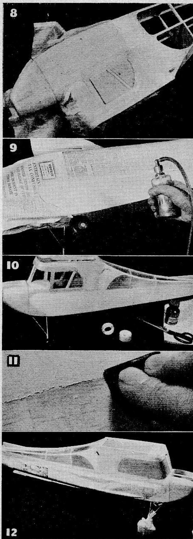
Fig. 8. Advantages of wet silk are most appreciated when covering rounded nose and cabin sections.
