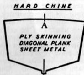
FIG. A (left) shows a typical hard chine cross-section.
