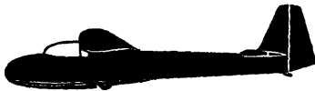
FIG. 2 (e). T. 42. Eagle 3. High performance Two-seater. Span 58 ft. Aspect ratio 14.8. Best gliding angle 1 in 31
