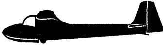
FIG. 2 (b). Skylark 2. Span 48 ft. Aspect ratio 16.0. Best gliding angle 1 in 30. Skylark 3 is similar, but has span 62 feet. Aspect ratio 20.5. Best gliding angle 1 in 36
