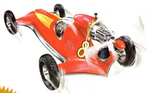
Zigs, zags, spins and spills. Free-running or tether. 12" high-impact plastic body. Aluminum chassis and wheels. Babe Bee .049 engine. Dubl-Tuf nylon prop.
