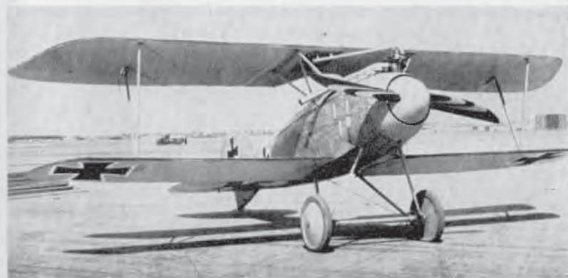
Albatros D III, fitted with D Va type rudder.
