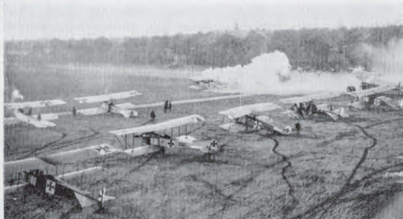
A varied collection of two-seaters at a German airfield in 1915. The aircraft are Albatros B IIs, Aviatik B Is and B IIs. (Photo: Imp. War Museum.)
