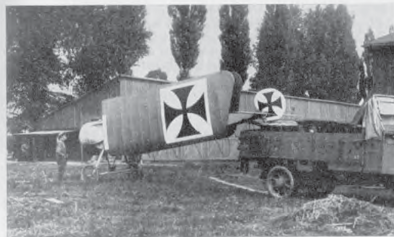
Fokker E I, (serial 36/15) folded for transport. (Photo: W. R. Puglisi.)
