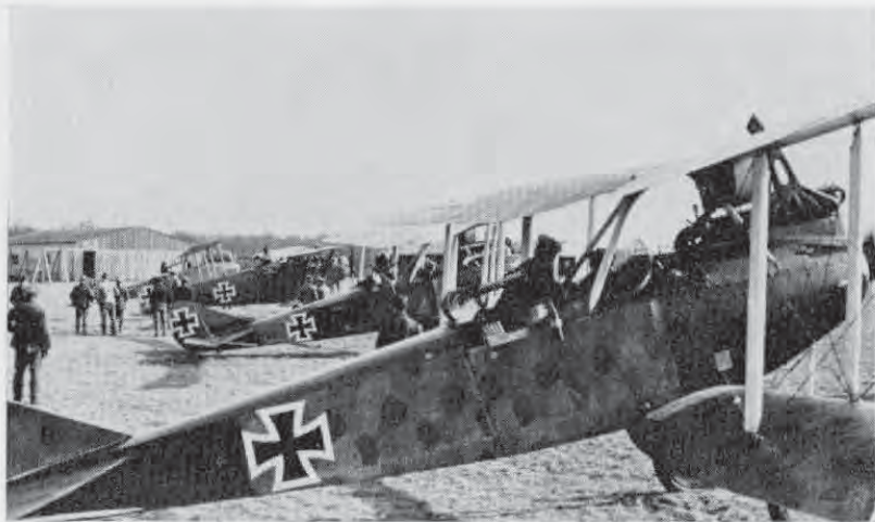
An interesting collection of two-seaters, typifying the equipment of 1917-18. In the foreground is a Rumpler C IV, the other aircraft being a Rumpler C VII, a Hannover CL IIIa and a D.F.W. C V. (Photo: A. Imrie.)
