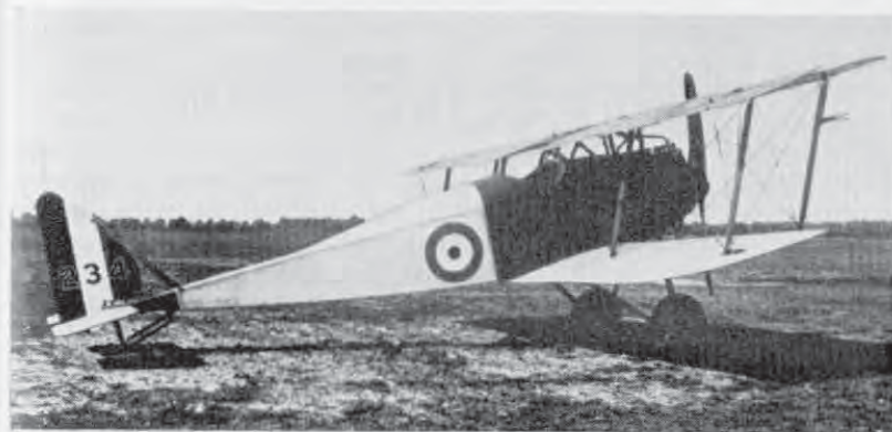
Halberstadt D III captured by the R.F.C. and given British roundels. (Photo: Aero Modeller .)
