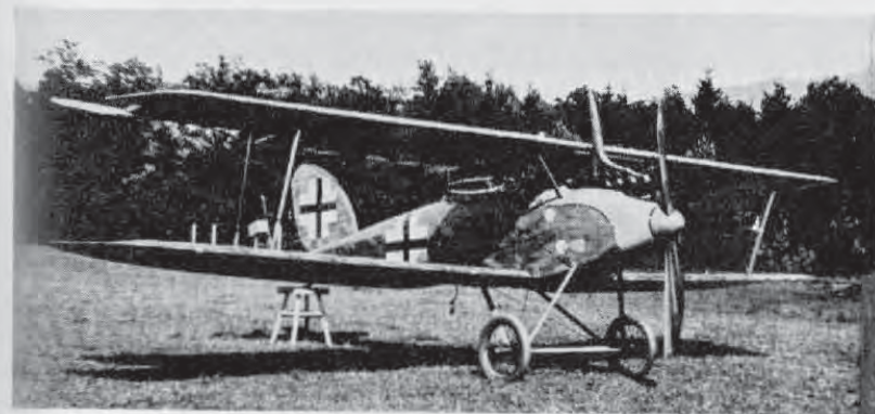
Halberstadt CL II, built under licence by B.F.W. Note vertical "rhino-horn" exhaust pipe.
