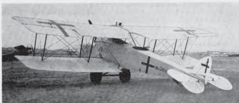
Albatros C III (licence-built by D.F.W. with modified fin and rudder). (Photo: A. Imrie.)
