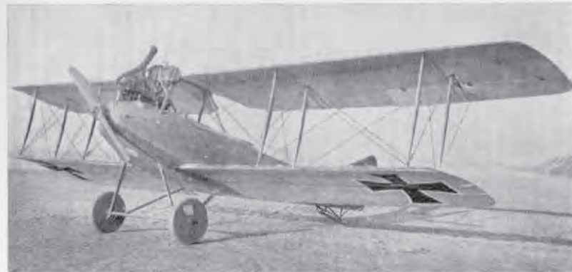
Albatros C Ia (licence-built by B.F.W. with 180 h.p. Argus). (Photo: A. Inrvie.)
