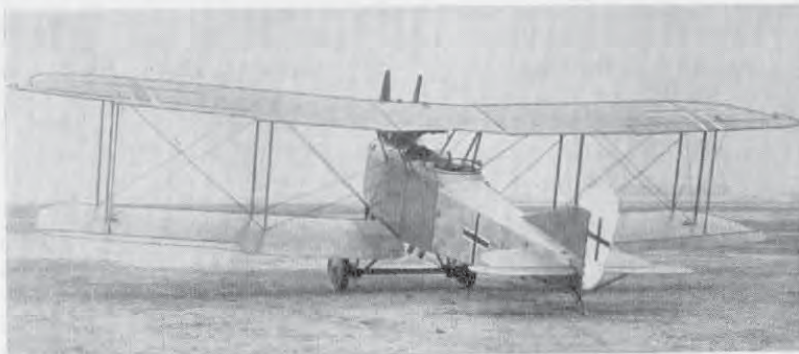
A.E.G. J II, with balanced control surfaces. (Photo: A. Imrie.)
