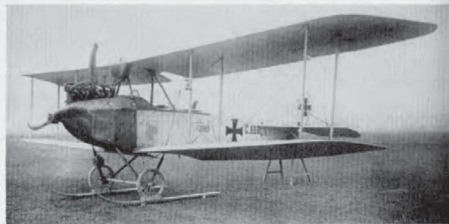
Rumpler C I with jury ski rig, (serial 6081/16). (Photo: A. Imrie.)
