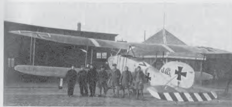
One of the specialised ground attack aircraft used in increasing numbers by the German Air Force from 1917 onwards—an Albatros J 1 (J 415/17). (Photo: A. Imrie.)
