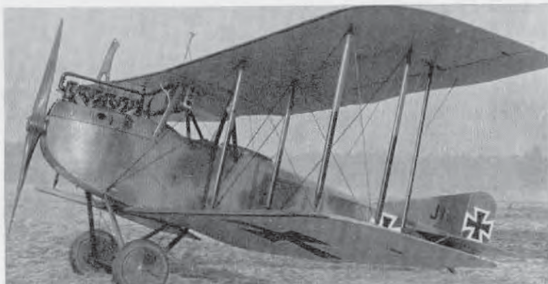
A.E.G. J Ia, with modified aileron link struts. (Photo: A. Imrie.)
