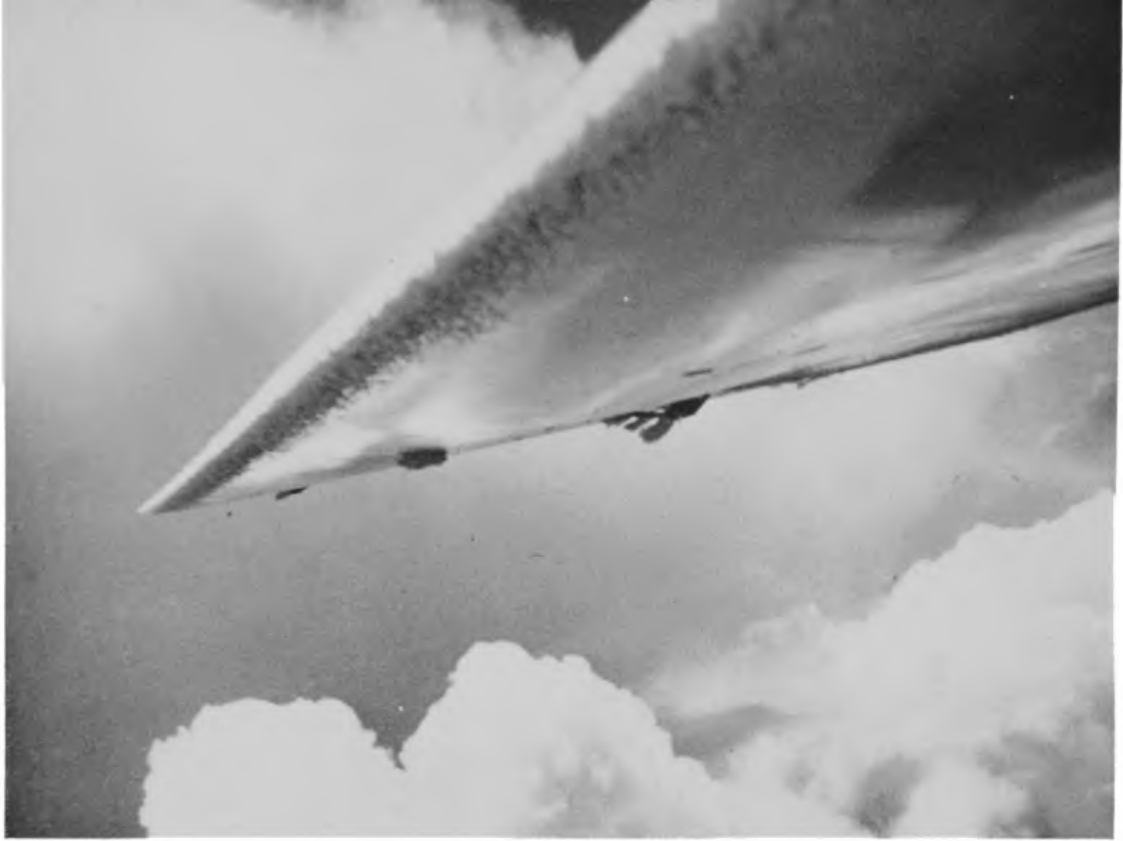
Light icing on the wing of a Skylark 2 (from a colour transparency by T. A. M. Bradbury)
