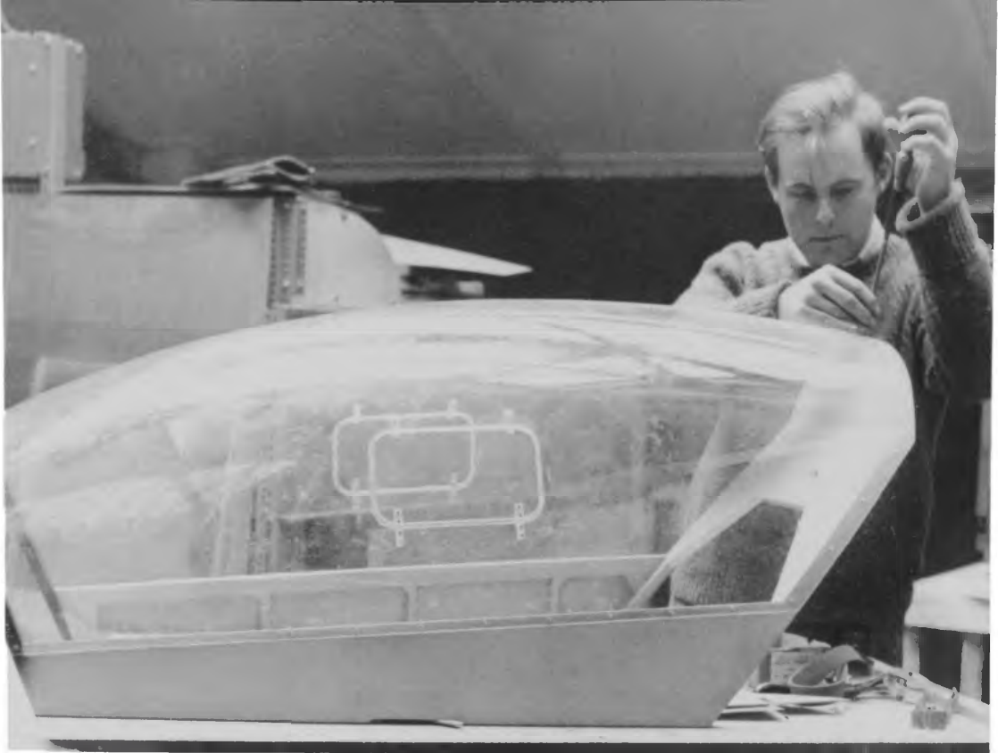
A moulded Perspex canopy for a Skylark 4 being fitted up by an expert in moulding technique (photo: Alex Watson)
