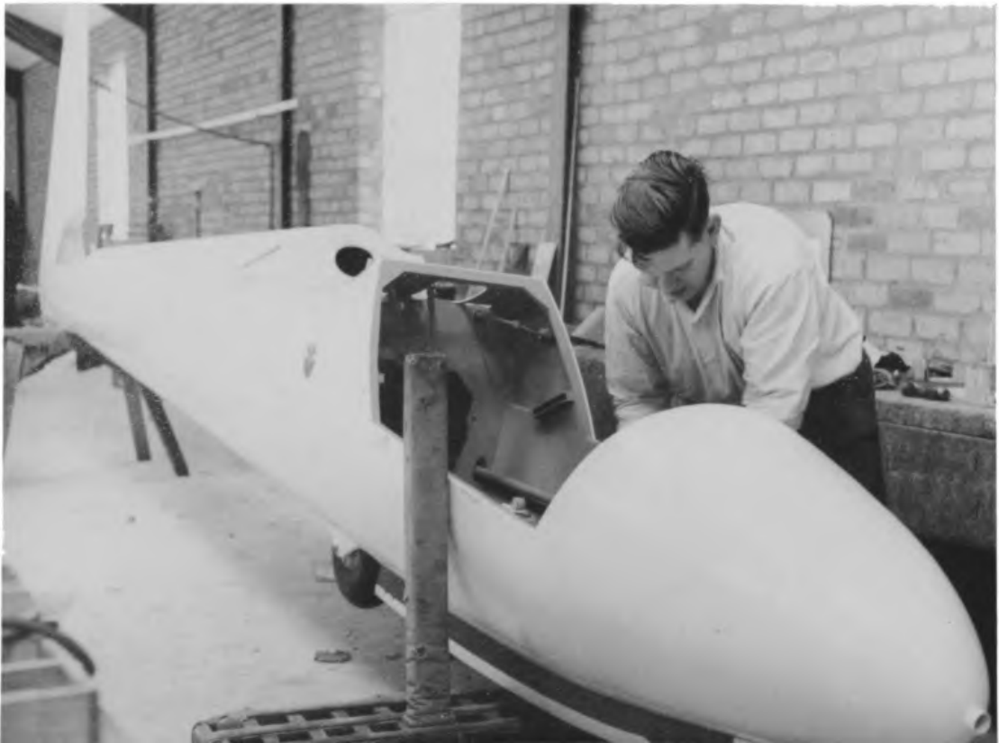
A Skylark 4 fuselage in the fitting-up shop (photo: Alex Watson)
