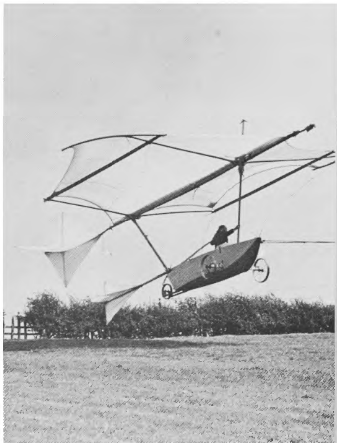
1 (a) Replica of Cayley's 1852 Riding Rudder glider, built by John Sproule; (b) & (c) Replica of Cayley's man-carrying glider of 1853, built by Ken Fripp and flown by Derek Piggott. It was just controllable by what became known as 'the influencer'
