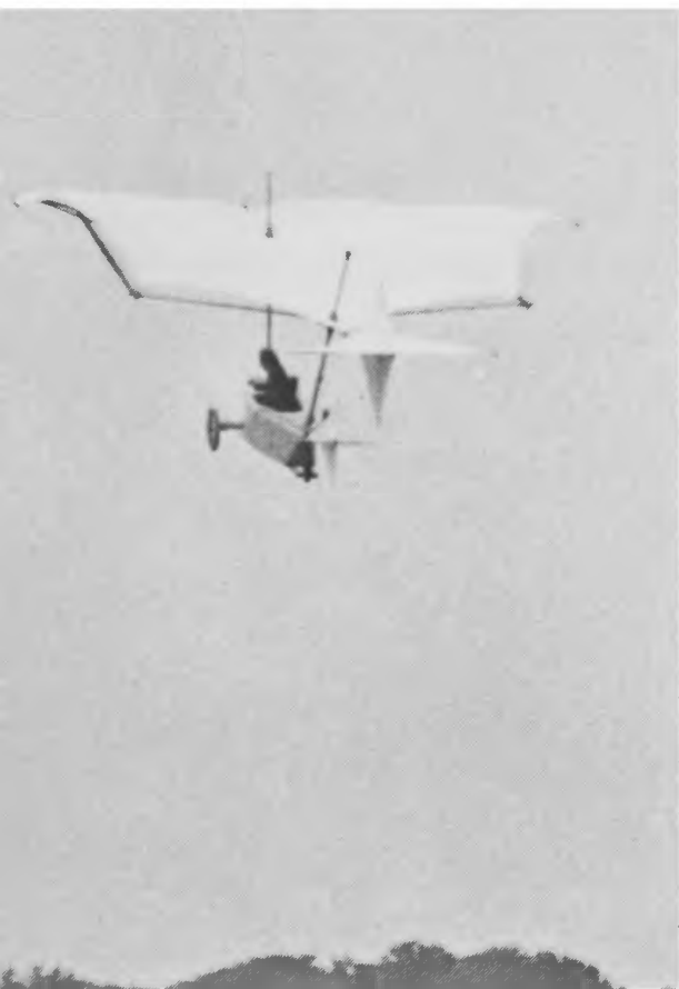
1 (a) Replica of Cayley's 1852 Riding Rudder glider, built by John Sproule; (b) & (c) Replica of Cayley's man-carrying glider of 1853, built by Ken Fripp and flown by Derek Piggott. It was just controllable by what became known as 'the influencer'
