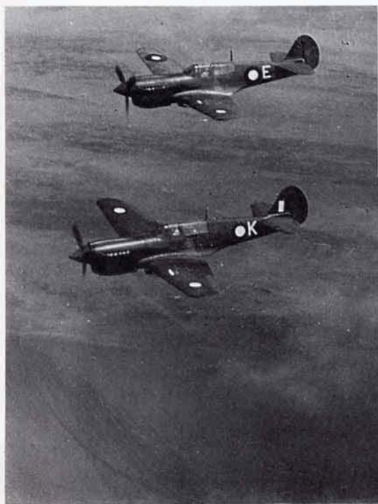
Below Mk. IV's of No. 84 Squadron, code LB-. Note variation in size and positions of roundels, all aircraft with dark green patches along leading and trailing edge of wings and tail plane and on fin and rudder on standard USAAF OD/grey scheme. LB-K probably A29-618. (AWM)
