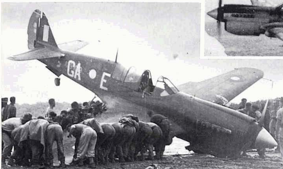
Left Mk. IV of No. 75 Squadron, RAAF with collapsed undercart probably due to burst tyre. Serial probably A29-1019 (via Frank F. Smith)
