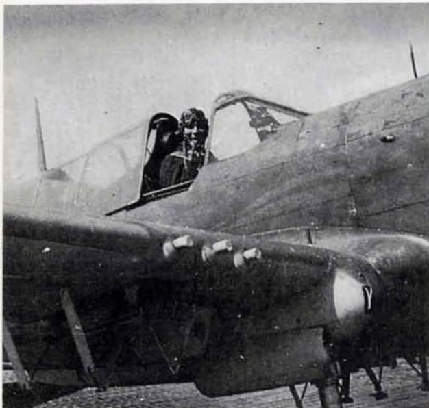
Detail shot showing wing guns, camera gun and bomb rack.
