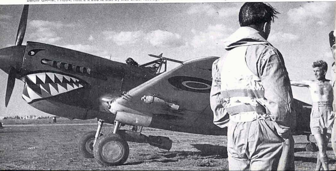
Below GA-M, FR864, note 2 x 250 lb side by side under fuselage and 4 x 40 lb bombs under wings. (IWM)
