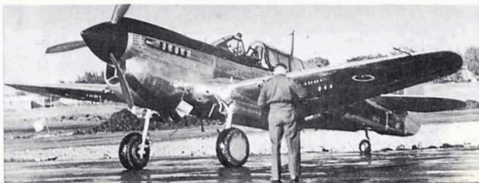
This Mk. III appears to be NZ 3119 stripped down to bare metal with black spinner and anti-glare panel. (via R. C. Jones)
