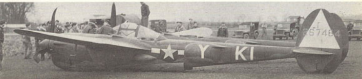
Below: P-38J of the 55th FS, belly landed at Kingscliffe, Northants. (Ray E. Bowers)
