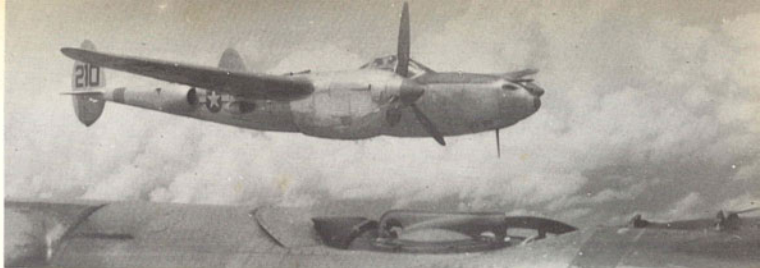
Above & below: Unusual pair of photographs showing a P-38J of the 18th Fighter Group first with starboard then with port engine dead and aircrew feathered, "Rickie Boy". (photos Peter M. Bowers)
