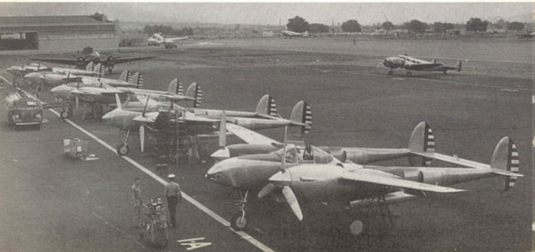
Line-up of natural metal P-38's, note cover plate on turbo-supercharger. (USAF)
