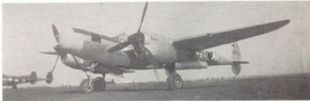
Right: P-38L 'Pathfinder' with BTO (bomb-through-overcast) radar in bulbous nose. Probably of the 67th Tac Recon Group, 9th Air Force, ETO.
