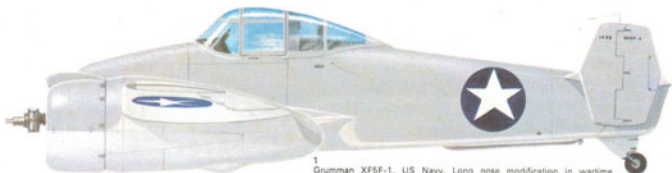
1 Grumman XF5F-1, US Navy. Long nose modification in wartime camouflage, post May 1941.
