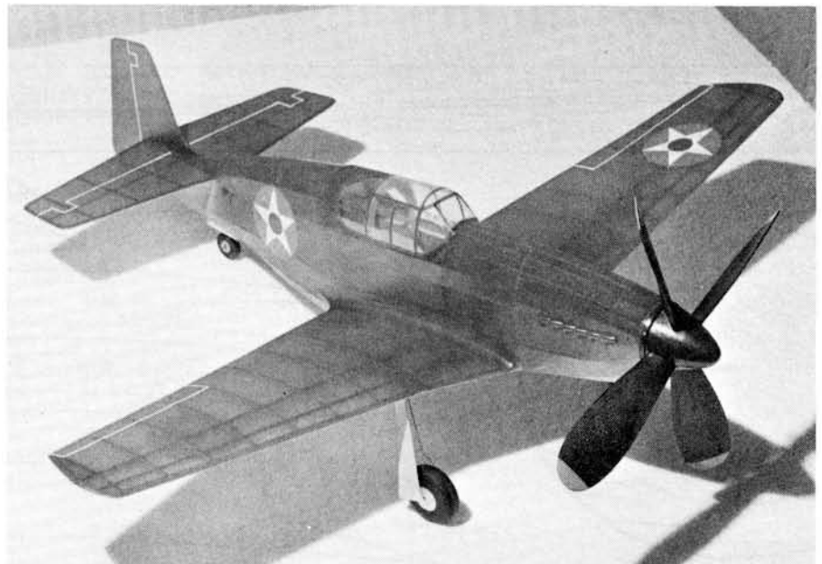
Blades of the big flying prop are built up from sheet stock and wet-shaped around a tin can. Colored tissue was used to help save all possible weight. Performance proves it paid off.
