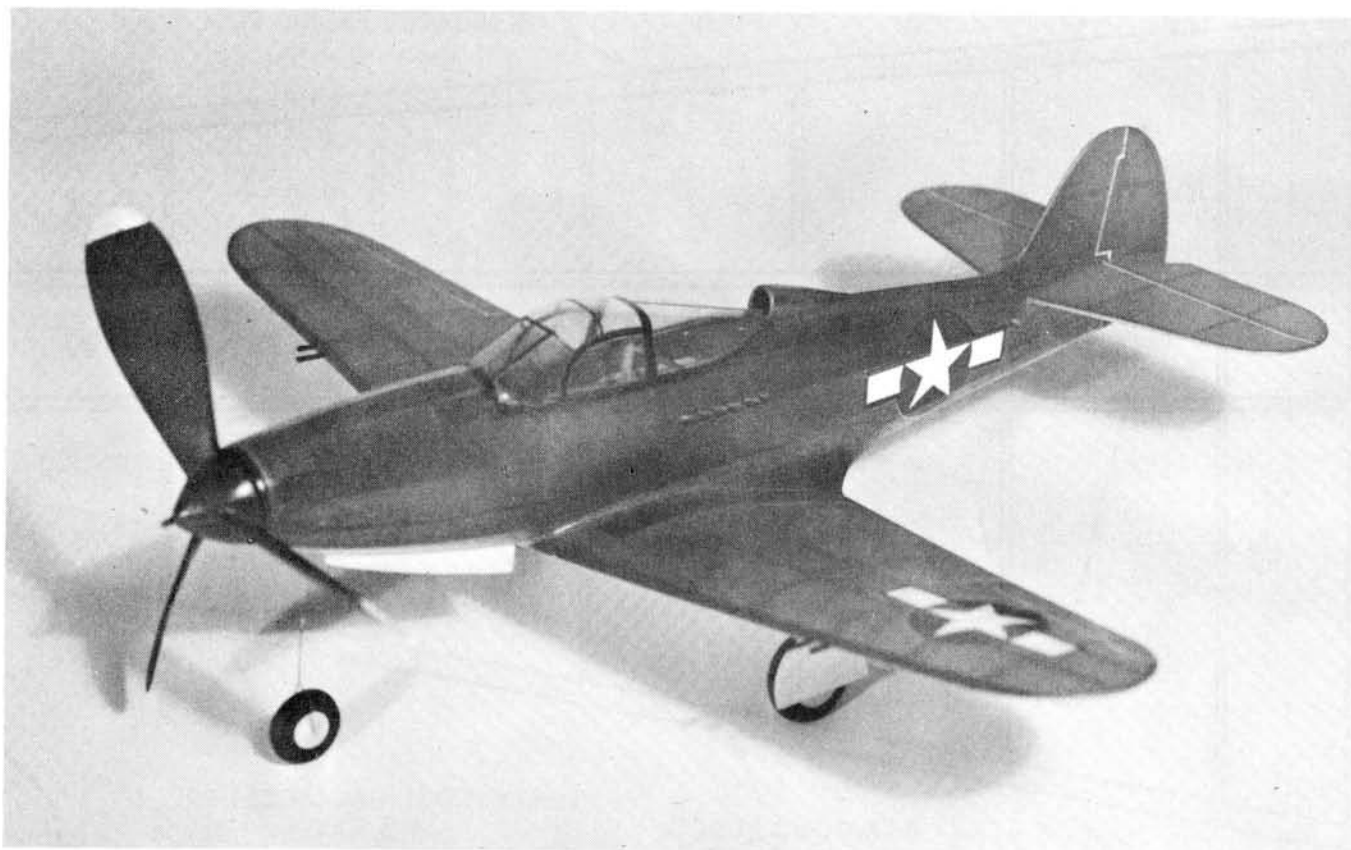
The author's Airacobra has put in many one-minute-plus flights. The long nose moment simplifies proper balancing, and the trike gear makes takeoffs pure pleasure.
