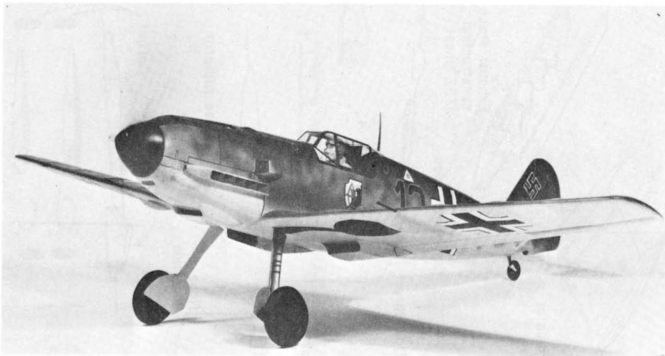
The characteristic splayed landing gear of the Bf 109E is very evident in this photo of the author's model. Markings are from the 8/J G.1., with yellow under-nose and wing tip undersides, and black "13" outlined in red.
