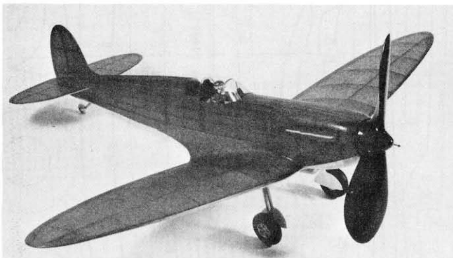
Note the generous blade area of the propeller in this photo of the Spitfire before the final finish was applied. Carving of balsa props for rubber power is covered on page 124.
