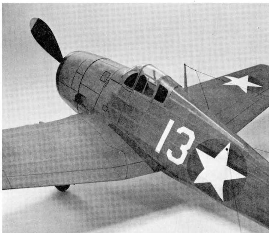
Bill's model of the Hellcat was covered with colored transparent tissue. The text explains how he got the two-tone effect of dark blue on top and light grey underneath. Lines are India ink.
