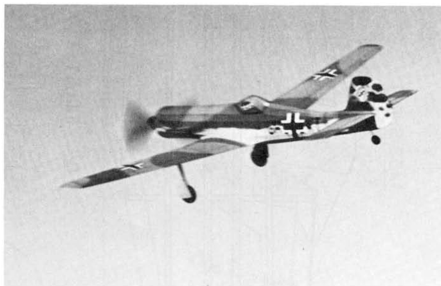
With its big prop scooping up large chunks of air, Hal's TA-152 is off for another flight. The long scale landing gear permits use of a very efficient flying propeller.
