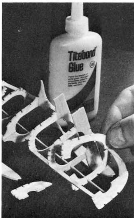
6. When dry, remove the construction from the plan and glue in place the opposite halves of the formers, carefully lining them up and ensuring absolute "squareness." Titebond Glue is recommended for all constructional work with balsa wood. It can be diluted slightly with water if desired.
