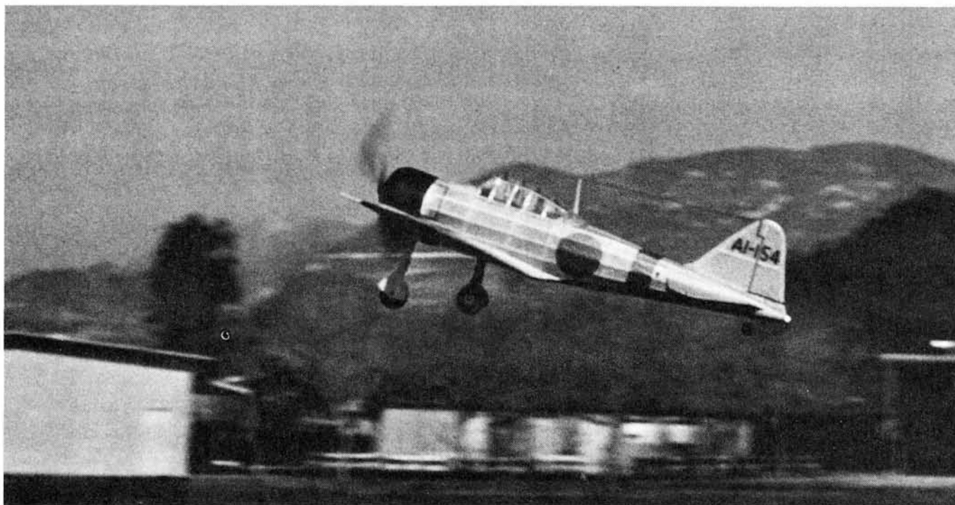
How's this for realism? Bob's Zero climbs out steadily after takeoff. Note two-bladed Kaysun prop used for flying. A seven inch prop cut down to six works best. Includes free-wheeling hub.
