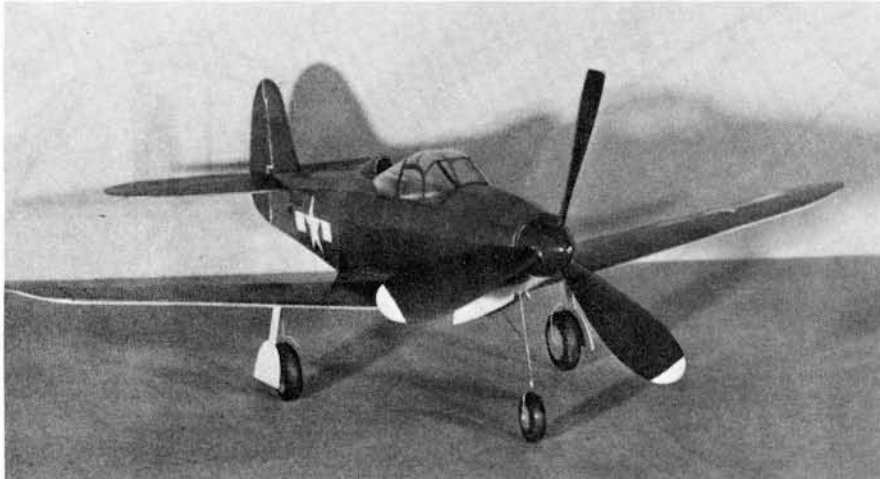
Hand carved three-bladed balsa prop was found to be more efficient than the popular plastic ready-made two-bladers.
