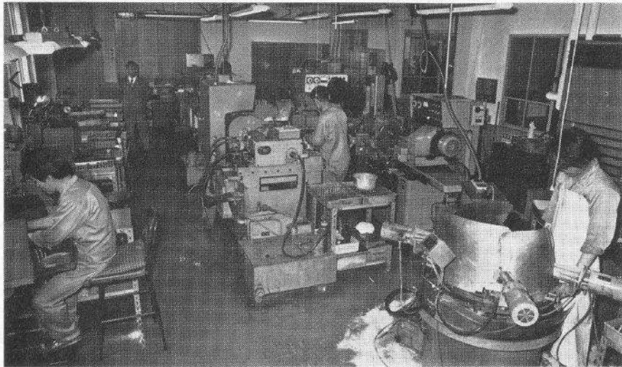
Machine shop engaged in mass production of components such as cylinders, pistons, wristpins and crankshafts, where a high standard of automation is used, and regular inspection of quality is maintained by personnel. A lot of the machinery has been specially designed and made by O.S.
