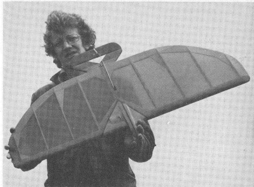
Vernon Hunt joined the ranks of the "big model" brigade—this design having around 390 square inches of wing area, tipping the scales at between 13 and 14 ounces. The leading edge is channel-sectioned for lightness, and spruce reinforced for strength. Root chord is nearly 12 in. wide while the span is 35 inches. He qualified for the 1975 European Championships with this model.
