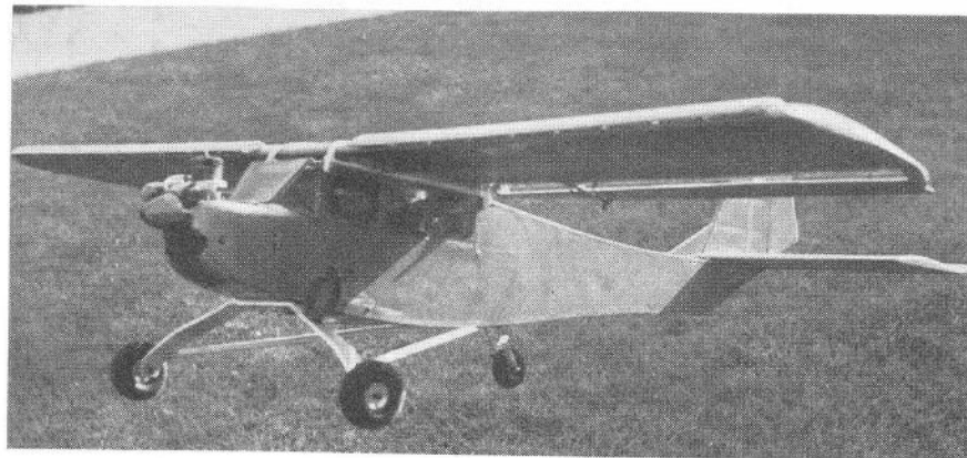
Martin Reed's second thoughts on Stol design. This one has a 54" span, Merco 35, full span L.E. slats, slotted flaps and ailerons.
