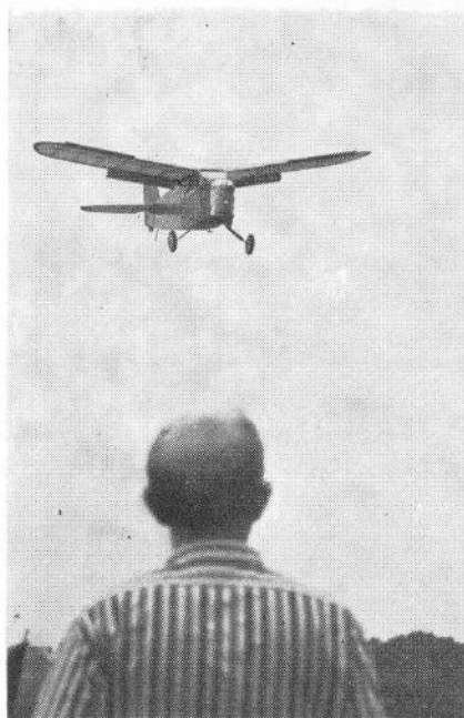
Stol Mk. 1 again, this time on finals with full 85 degree flap setting. Although in level attitude, model is in fact descending steeply, very near to the stall with engine at about one-third power.
