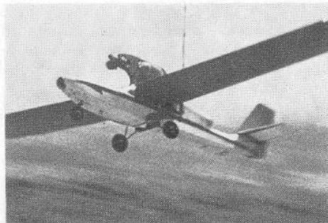
The Wavemaster takes off at an all-up-weight of some 20 lb. Model had a level speed of about 60 m.p.h.
