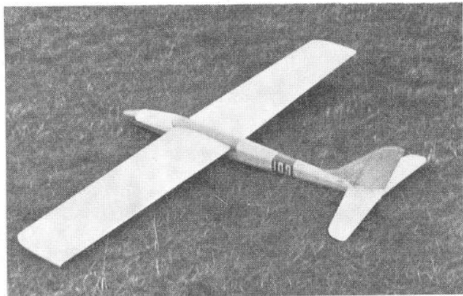
Right: Sleek 'Phase Four' design by top glider aerobatic pilot Chris Foss has slim fuselage for minimum drag.
