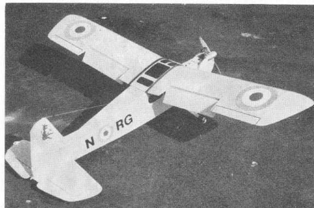
J. Stennard's 'Super' Super 60 incorporates all 'Straight & Level' modifications, but also has large area 60 degree plain flaps. Uses O.S. 40 engine.
