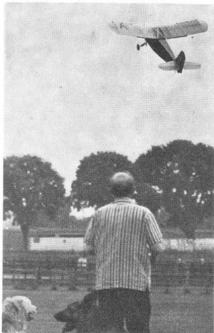
Writer's 'Stol Mk. 1' demonstrates vivid short take off and steep climb out, using optimum 20 degrees take-off flap setting 48 in. span, three pounds weight, O.S. 19 engine heavily muffled.
