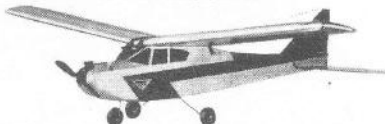
GYRON 36" Wingspan model featuring all sheet construction. For 049 Glowmotors and Rudder only control.
