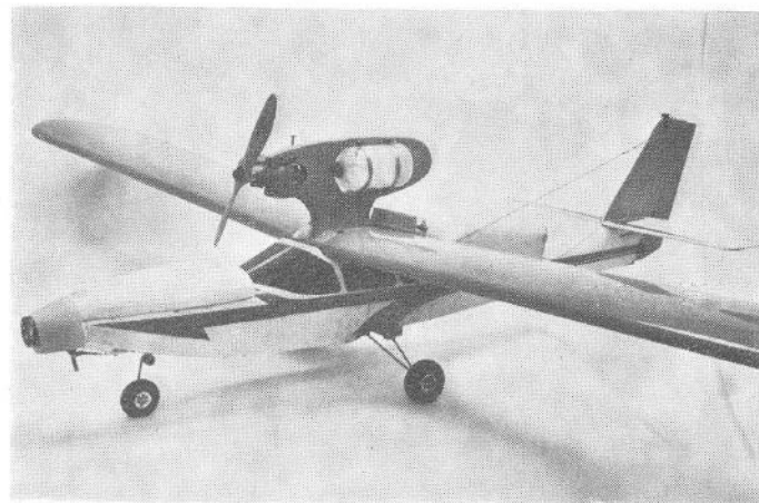
The Wavemaster after modifications to take the RPV equipment. Note the TV camera mounted on nose. Power pod was stripped to take larger fuel tank.
