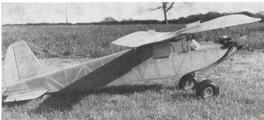
R. M. Pilgrim built this Super 60-based Stol which has D.F.S. type airbrakes as well as large area, 85 degree split flaps. Very 'Stol' but some control problems at ultra-low airspeeds. Note bracing wire, highly recommended by author.
