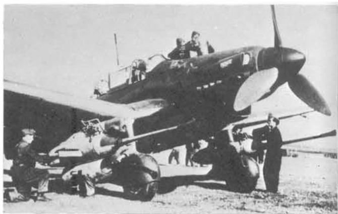
33. The Ju87G tank-buster, with two BK 3,7 Flak 18 cannon, proved extremely effective in its specialised rôle on the Russian Front. (Author's collection)
