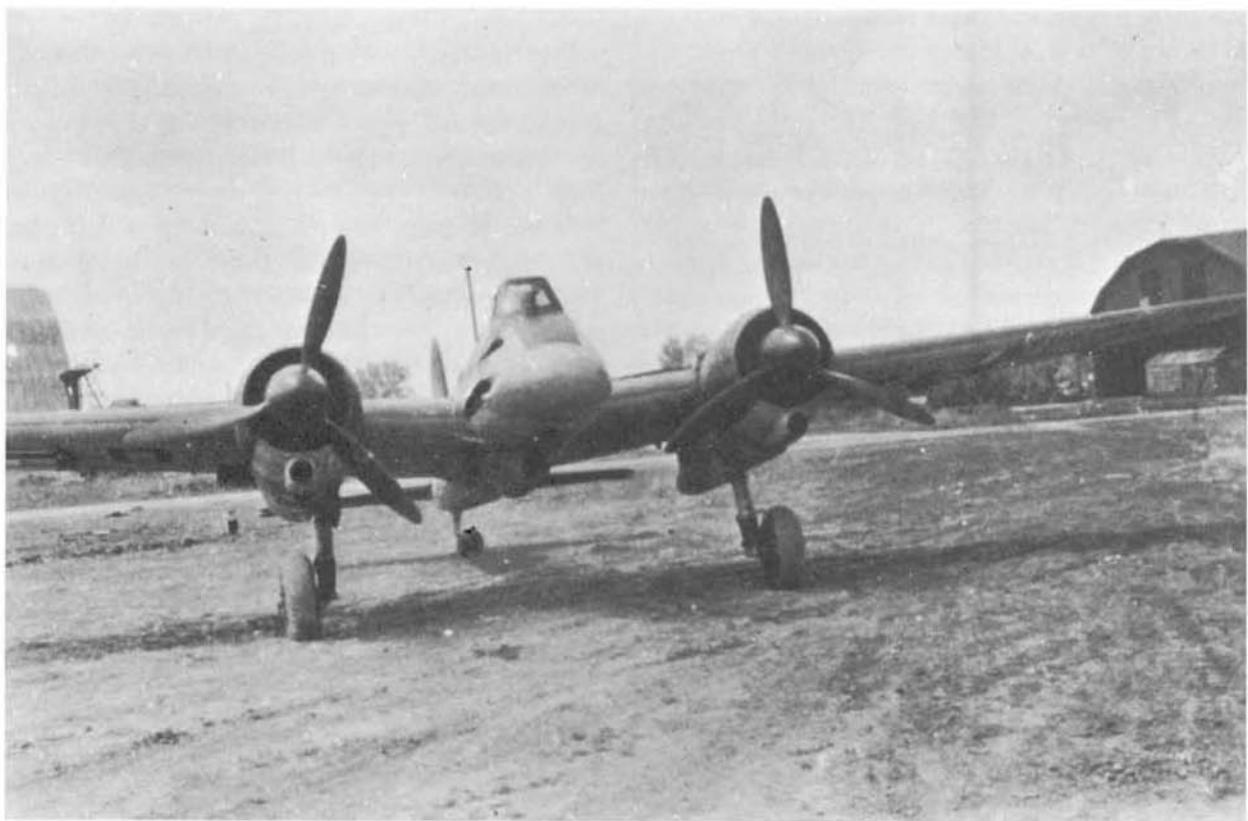
20. Front view of a yellow-nosed Hs129B-1/R2, showing the 30 mm MK 101 cannon beneath the fuselage. During the Soviet advance of November 1942 pilots of 8/Sch.G 1 often went into action without proper training for anti-
