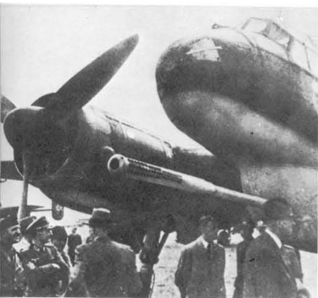
25. The electro-pneumatically operated 75 mm PaK 40 cannon fitted to a Ju88P-1 for anti-tank operations, late 1943. A small test batch became operational under the Führer der Panzerjäger with Panzerjäger-Staffel 92, but although the cannon was effective the aircraft lacked manoeuvrability. Earlier attempts by III/KG 1 to operate 75 mm cannon-equipped Ju88s independently resulted in the unit's destruction. (Author's collection)
