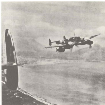
36. Messerschmitt Bf110D-3s of I/ZG 26 (note wing-mounted 198 Imperial gallon drop-tanks) operating over Greece in summer 1941. (Bildarchiv)
