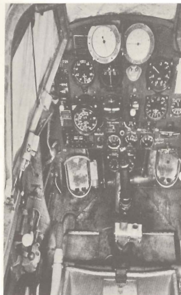
10. The cockpit of the Bf109E—after modifications by its British captors, including the removal of the reflector gunsight and the fitting of a new airspeed indicator. The cockpit of the little 'Emil' was cramped even for a man of average build. (Imperial War Museum)
