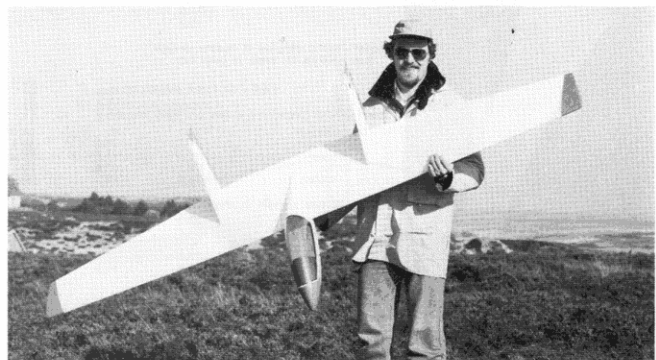
Left, Roland Sommer was third with his Vampir, weight 1.4 kg., has Roland's own aerofoil and employs separated elevator and ailerons.
