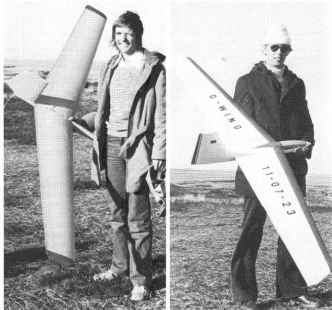
Far left. Winner Jurgen Landscron with his swept-forward entry. Eppler 182 aerofoil, 1.85 kg. weight and separated ailerons and elevators, data at right.
