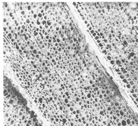
Photo 2: Electron microscope photograph of typical cross-section of balsa wood. Magnification 200 times full size. Note hexagonal cell structure, with rectangular cells in growth rings.
