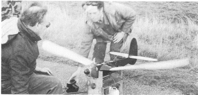
John Drake (left) assisted by Roy Sturman of Autogyro fame. The wing is beating at three beats to the second!! Exposure 1/25 second. Blurred wing illustrates the high flapping rate. There is no need to hold the fuselage, the characteristic St. Vitus' Dance of most ornithopters has been overcome by articulating the wing.
