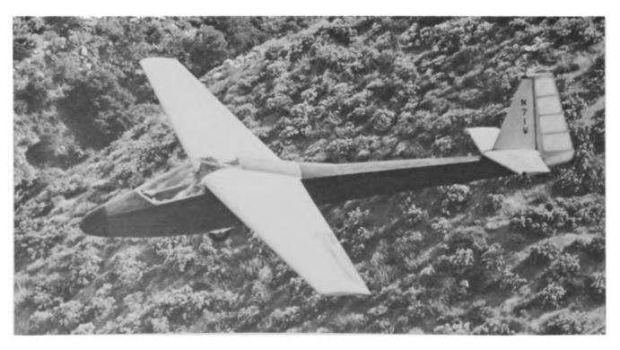
The Tern is a single-seat sailplane with a good performance and simplified construction, designed by Terry Miller for home-builders. Many are under construction in the USA and plans for the aircraft have been sold throughout the world. The Tern 2 is an improved version of the Tern 1, with increased wing span and a drogue parachute fitted in the base of the rudder. The prototype Tern first flew in September 1965, and the Tern 2 made its first flight three years later, in August 1968.
