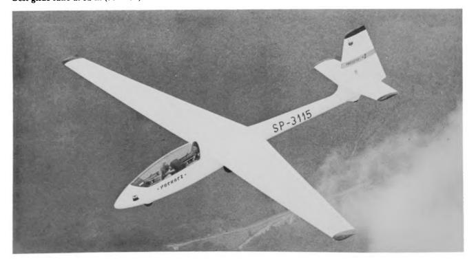
The IS-28B2 is an improved version of the 15-metre IS-28, the two-seat high-performance sailplane designed by Dipl. Ing. Iosif Silimon and his team, from which it differs primarily in having 17-metre span all-metal wings, a longer and more slender fuselage and reduced wing and tailplane dihedral. The original IS-28, which first flew in August 1970, had a glide ratio of 25 and minimum sink speed of 0.85 m/sec (2.79 ft/sec).
