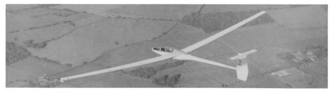
wing loading and low drag should give a high lift/drag ratio at high speeds. The braking system is operated by lowering the camber-changing flaps and raising the spoilers on the upper surfaces to control the speed.
