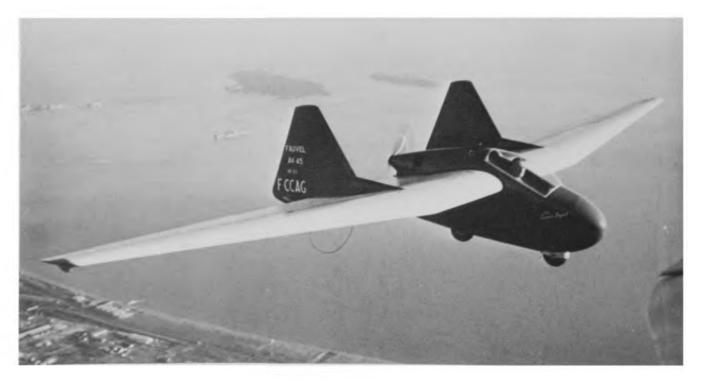
The AV.222 side-by-side two-seat tailless motor glider is a lighter and simplified version of the AV.221; both are derived from the AV.22 tailless sailplane. The AV.222 is
